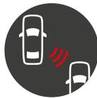
We've further improved our Blind Spot Information System (BLIS). It now uses radar technology to alert you to vehicles closing up in your blind spot. There's also Cross Traffic Alert, which watches out for vehicles you can't see when you're reversing out of tight parking spaces.
