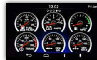
*Pre-loaded virtual gauges include oil temperature, transmission temperature, manifold boost, present and average fuel economy, DPF status and engine torque.*
