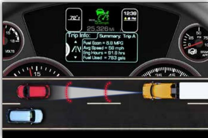
Adaptive cruise control (ACC) can make driving trucks safer and less fatiguing. Integrated with your normal cruise control system, ACC “reads” traffic conditions via front-facing radar sensor and modulates the throttle and the brakes to keep your truck at a pre-set distance from the vehicle in front of it. Then, when the road is clear, the system will re-accelerate the vehicle back to the set speed.
