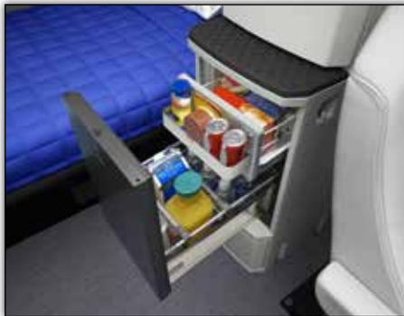
*Large capacity, drawer-style refrigerator/freezer mounted at mid-level for wide open access without bending over.*
