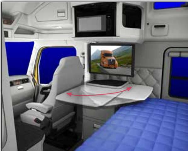
*To maximize stand-up room in the sleeper, a pull of the latch unlocks the table which may be rotated 90 degrees above the bunk, also giving you easy access to the drawers below.*
