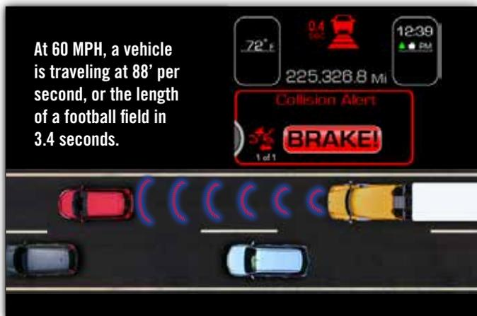
At 60 MPH, a vehicle is traveling at 88' per second, or the length of a football field in 3.4 seconds. Far beyond a mere warning system, Kenworth collision mitigation detects when the truck may be about to collide with another vehicle or object, alerts the driver and takes pre-emptive braking action — when necessary — to avoid or considerably reduce the severity of a crash.
