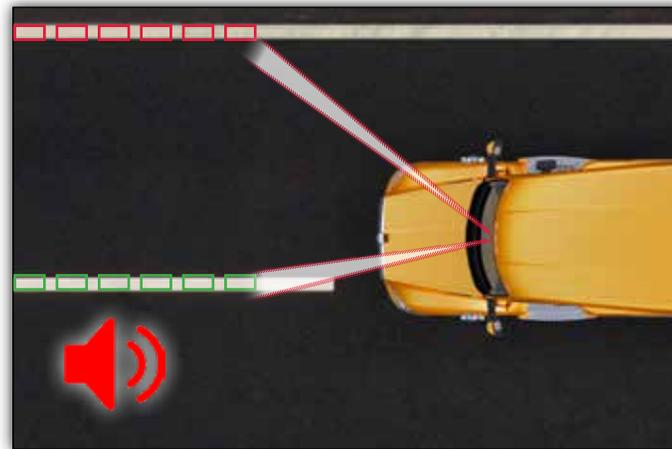
Kenworth's lane departure warning system helps combat lane drift due to fatigue and distractions. The system continually monitors the truck's location related to lane markings and automatically emits a distinctive audible warning whenever an unintended lane change (unsigned) is detected — alerting the driver to make a correction.
