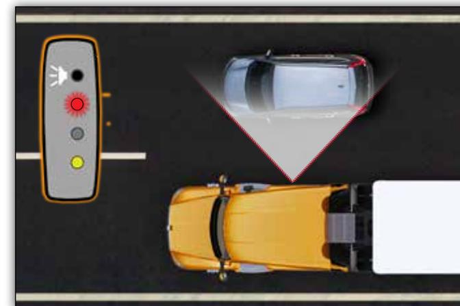
The side object detection system continuously monitors a truck's blind spots and provides the driver with audible and visual alerts when an object or vehicle has entered these zones — invaluable when making a lane change or negotiating tight delivery sites.
