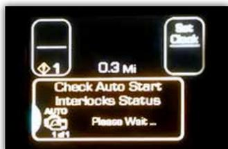
*The system automatically starts the engine if batteries run too low or the engine becomes too cold, then turns the engine off once conditions have met preset parameters — a smart way to manage off-duty charging requirements without idling the truck unnecessarily.*
