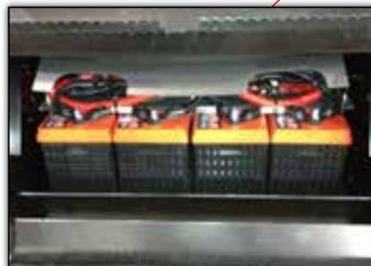
*Four Group 31 batteries, electrically isolated from the truck, power the system.*
