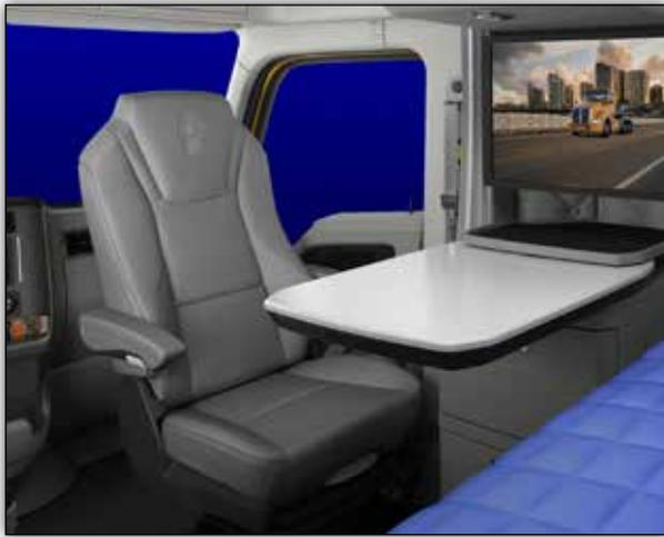
*The Drivers' Studio includes the 180-degree swivel passenger seat and swivel table option set, which maximizes the driver's living space by combining the cab and sleeper into a large studio, allowing the driver to relax in comfort in the passenger seat rather than being confined only in the back of the sleeper. It also allows for viewing of the TV from the passenger seat or the bunk.*
