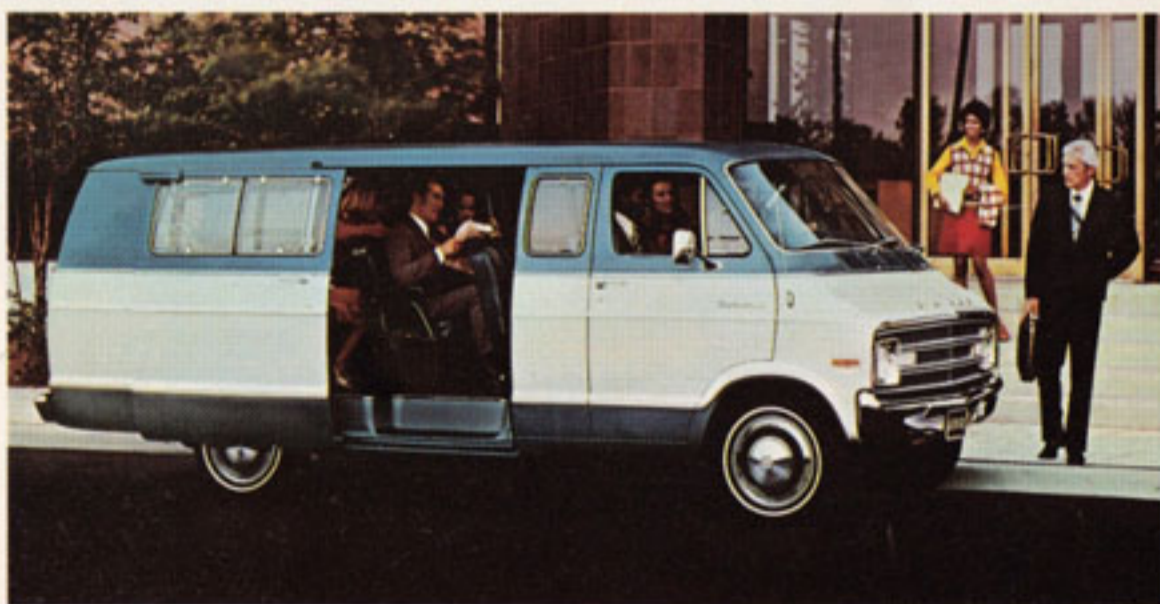
Maxiwagon. Its 212-inch overall length allows room inside for four bench seats, in addition to driver and front passenger seats, so that up to fifteen adults can ride in comfort. Available in two models, B200 and B300.
