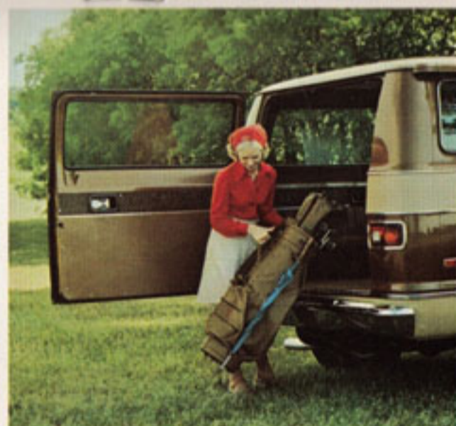
Full-width rear door, standard for rear loading convenience. A door check holds it open; big window adds to rear visibility.
