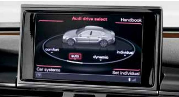
**Audi drive select** | Exclusive to Audi, this system provides advanced control of the vehicle's steering, transmission shift characteristics and engine response. The system offers drivers the ability to configure vehicle drive characteristics exactly to their liking with the choice of Comfort, Auto, Dynamic or Individual settings.
