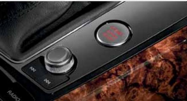
**Keyless Start** | With the touch of a button, the driver can start/stop the engine without removing the key from a pocket or purse.
