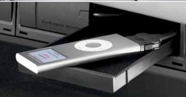
**Audi music interface** | This connective technology offers intelligent integration with the iPod® and iPhone®. Any iPod® Generation 4 and higher may be connected, providing full iPod® controls on the MMI® screen. This feature allows connection of a USB flash drive or a conventional auxiliary audio input as well.
