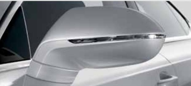
**Auto-dimming, power-adjustable and manual-folding exterior mirrors** | Exterior mirrors with automatic dimming recognize glaringly bright headlight beams behind the car and darken the mirror glass automatically. In addition to being electronically adjustable, the manual-folding feature helps protect the mirrors by collapsing them inward to fit in tight spaces.
