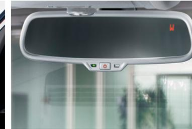
Auto-dimming interior rear view mirror with digital compass
