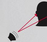
Unlike with high-frequency sounds, the brain cannot detect where low bass frequencies are coming from, making it seem as if the sound is hitting both ears at the same time. Because of this, Bang & Olufsen® sound engineers only had to design one custom-fitted subwoofer to reproduce the kind of deep, cabin-filling bass that brings music to life.
