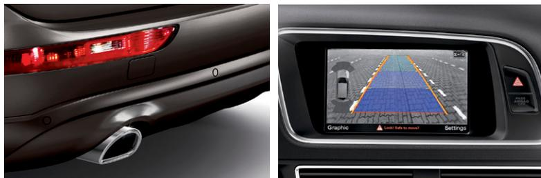
Parking system plus with front and rear acoustic parking sensors    Parking system plus with rear view camera
