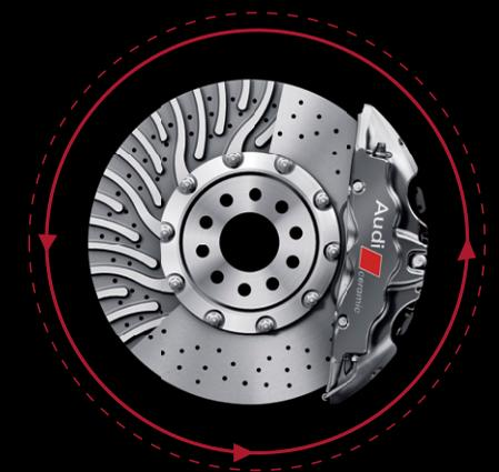
carbon ceramic rotor<sup>1</sup> // reduces rotational weight by up to 8.82 lb each, compared to traditional rotors
