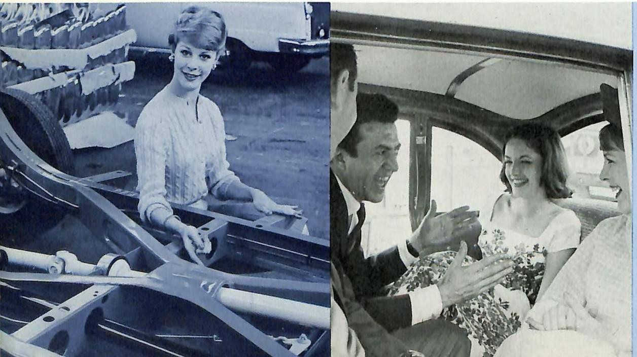
**EXTRA-RUGGED BODY.** The double channel X-frame is the sturdiest money can buy. A Checker is built to last. A Checker is *rattle-free* because live rubber body mounts are used in fusing the body to the frame. A Checker is *shock-proof* because the body is bolted to the frame, creating a more rigid unit than is possible with other types of construction. A Checker is *safer* because of heavy, double-wall construction.
