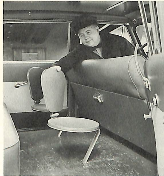
Checker exclusive! Auxiliary seats provide seating for two extra people; fold away when not in use.
