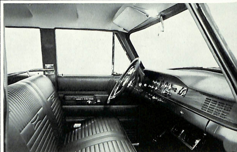
Three extra passengers sit on big, square, forward-facing auxiliary seats in the Checker A-12E Marathon Deluxe Sedan. Seats fold away when not in use.
