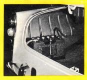
Rear Mounted Battery. Many operators now prefer the rear mounted battery option since engine heat frequently will affect length of battery life. Counter-balanced trunk lid is standard equipment.
