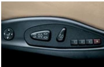
**Eight-way power front seats** includes **driver’s seat and mirror memory system**, which lets up to three drivers set their preferred seat and exterior mirror positions. Plus, the passenger’s-side mirror tilts down when vehicle is shifted into reverse gear. (330Ci; optional and included in 325Ci Premium Package. Lumbar support [shown] is included in 330Ci and 325Ci Premium Packages)
