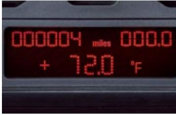
An **on-board computer** offers valuable travel information, with readouts on expected travel range on remaining fuel, average mpg and average speed. An external thermometer sounds a warning when the temperature falls below 38°F – indicating that the road may ice up.
