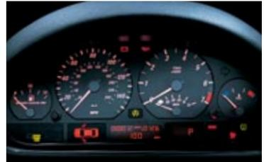
The **instrument panel** presents all important information at a glance through analog gauges and LCD readouts. When parking lights or headlights are on, the gauges are lit in an easy-to-read red.
