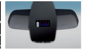
■ Rain sensor uses infrared light to measure the amount of rain. When the wipers are in the "intermittent" mode, the rain sensor automatically adjusts the windshield wiping interval as needed. Automatic headlight control (not shown), included with rain sensor, activates headlights by means of a sensor that responds to darkness.
