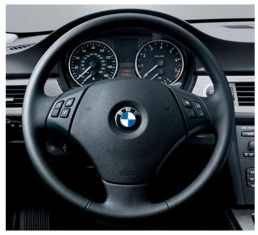
■ Three-spoke leather-wrapped multi-function steering wheel lets you keep both hands on the wheel while adjusting various comfort functions, such as changing the radio, CD selections and volume. Optional Voice Command (included with optional on-board navigation system) can be used to change radio stations and audio selection, navigation system destinations, and (accessory) telephone entries.
