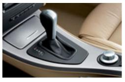
□ 6-speed STEPTRONIC automatic transmission provides a choice of three modes: "Drive," which incorporates BMW's Adaptive Transmission Control; "Sport" automatic, for a more dynamic shift pattern; and STEPTRONIC automatic, for the hands-on control of a manual without using a clutch. (Shown with iDrive, which is included with optional on-board navigation system)
