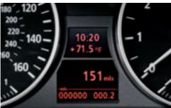
■ The **on-board computer** with Check Control provides valuable feedback on the vehicle's operating status: oil level indicator, distance to next service appointment and oil change, front/rear brake pad and brake fluid status, state emissions inspection due date, and other detailed information like spark plug and micro-filter status. It also provides travel information such as travel range on remaining fuel, external temperature, and more.
