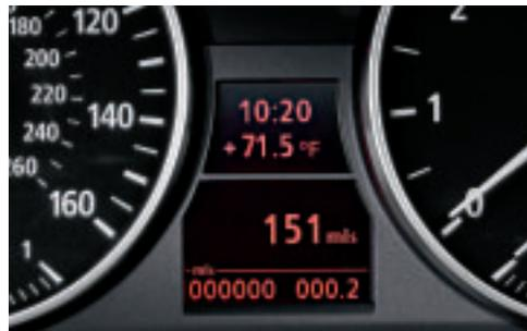
■ The **on-board computer** with Check Control provides valuable feedback on the vehicle's operating status: oil level indicator and distance to next service appointment/oil change, as well as other detailed information, such as spark plug and micro-filter status. It also provides travel information – travel range on remaining fuel, external temperature, and more.
