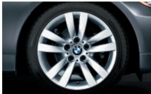
□ **Double Spoke (Style 161) light-alloy wheels and run-flat<sup>1</sup> performance tires.**<sup>2</sup> In front: 17 x 8.0 wheels and 225/45R-17 tires; in back: 17 x 8.5 wheels and 255/40R-17 tires.<sup>3</sup> (included in 328i Sport Package; opt. in 328xi, requires optional Sport Package)
