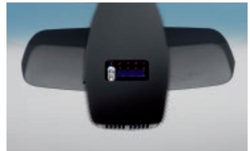
■ **Rain sensor** uses infrared light to measure the amount of rain. When the wipers are in the "intermittent" mode, the rain sensor automatically adjusts the windshield wiping interval as needed.
