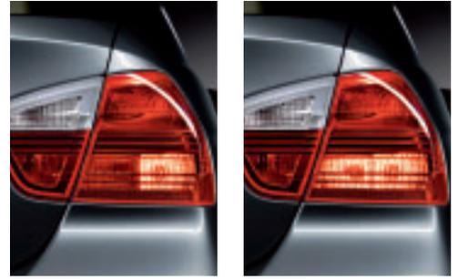
■ **Adaptive Brake Lights** increase vehicle visibility and signal the intensity of your braking action.
