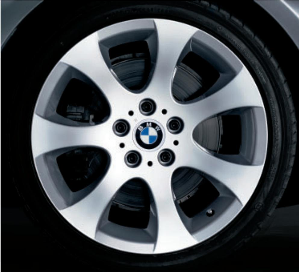
□ **Star Spoke (Style 162) light-alloy wheels and run-flat<sup>1</sup> performance tires.**<sup>2</sup> In front: 18 x 8.0 wheels and 225/40R-18 tires; in back: 18 x 8.5 wheels and 255/35R-18 tires.<sup>3</sup> (included in 335i Sport Package; opt. in 335xi, requires optional Sport Package)
