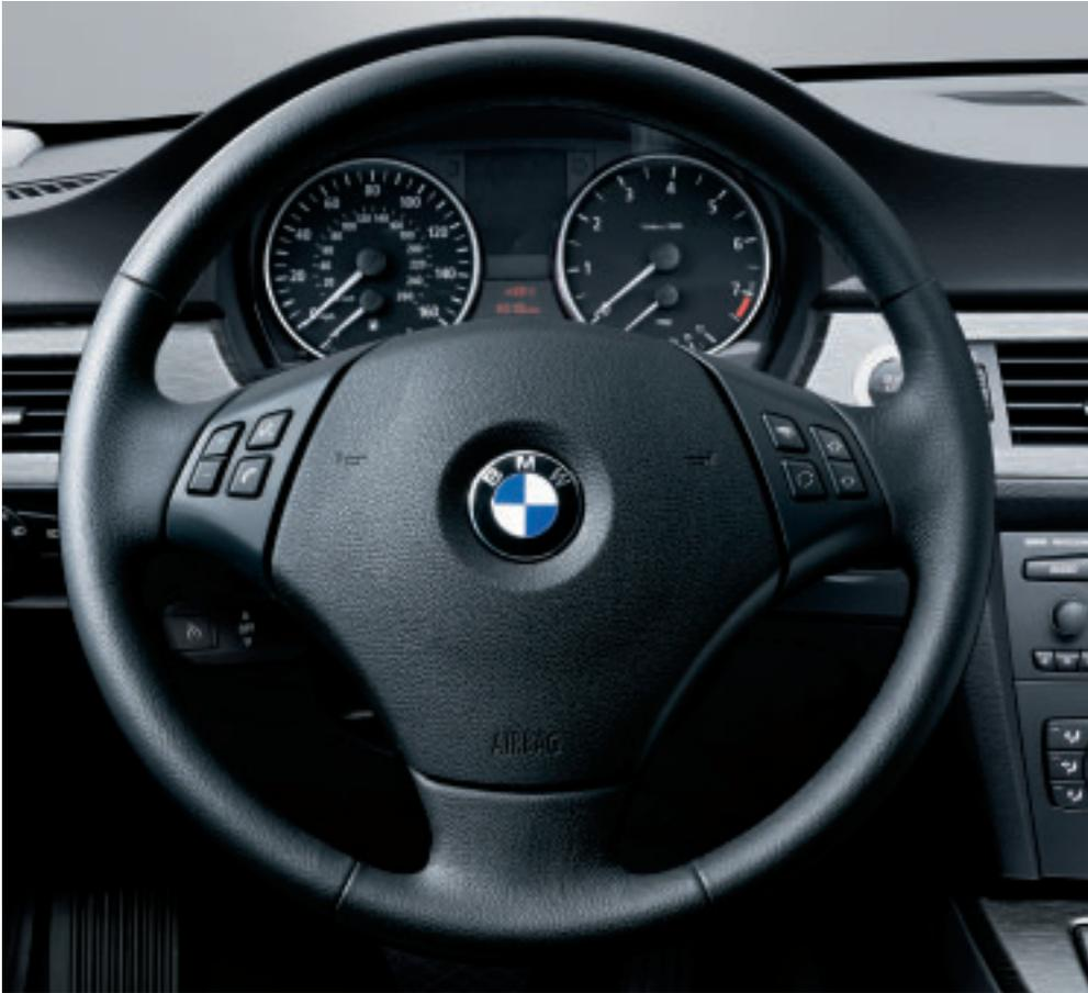
■ **Three-spoke leather-wrapped multi-function steering wheel** lets you keep both hands on the wheel while adjusting various comfort functions, such as changing the radio, CD selections and volume. Optional Voice Command (included with optional on-board navigation system) can be used to change radio stations and audio selection, navigation system destinations, and voice dialing of the telephone.
