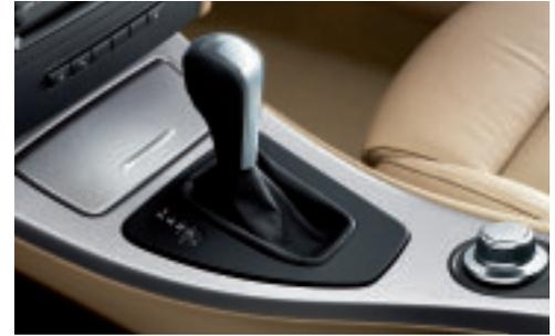
□ **6-speed STEPTRONIC automatic** provides a choice of three modes: "Drive" with Adaptive Transmission Control; a more dynamic "Sport" mode; and STEPTRONIC automatic, for the hands-on control of a manual without a clutch. The 335i with Sport Package includes steering wheel paddle shifters. (shown with iDrive, included with optional on-board navigation system)
