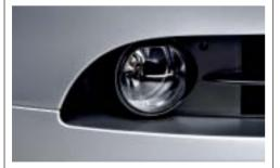
■ Halogen free-form foglights, integrated into the deep front spoiler, enhance your margin of safety in bad visibility. Ellipsoid free-form technology ensures even light distribution on the road.
