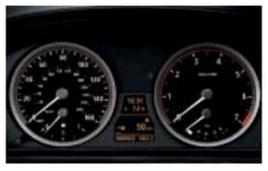
■ Easy-to-read **Information Display** with precise, dazzle-free analog indicators. Data, such as trip mileage counter, can be checked using LCD displays on the instrument panel.
