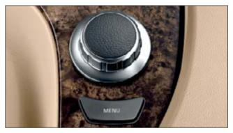
The iDrive Controller, which is conveniently located on the center console, allows you and your passenger to access and tailor many comfort features.
