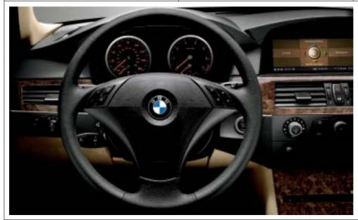
■ 3-spoke leather-wrapped multi-function steering wheel lets you keep both hands on the wheel while adjusting various comfort functions, such as changing the radio, CD selections and volume. Optional Voice Control (included with optional on-board navigation system) can be used to change radio stations and audio selection, navigation system destinations, and (accessory) telephone entries.
