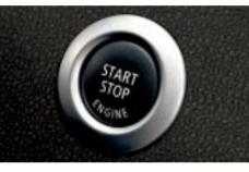
■ Engine start/stop button is a convenient method to control the engine. Simply insert the electronic identification fob into the starter switch slot and press the start button. Pressing the button while the engine is running will stop the engine.
