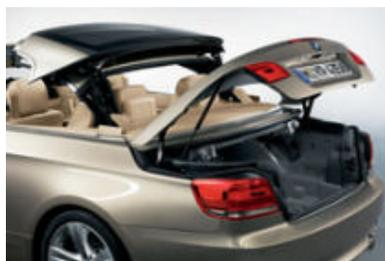
□ **Comfort Opening and Loading** feature (included with optional Comfort Access) offers a quick, easy way to stow and remove luggage or large packages from the trunk when the top is down. Simply press a button on the remote key to raise the hardtop up and out of the trunk and "freeze" it in position; another press neatly lowers the hardtop back into the trunk.
