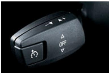
■ **Dynamic Cruise Control** lets you store and keep to a chosen speed above 20 mph, automatically applying the brakes on a downhill. It is activated via the left-hand steering column switch and deactivated by applying the brakes or via the switch.<sup>3</sup>
