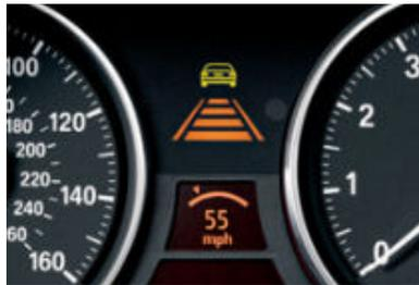
□ **Active Cruise Control** system uses radar measurements to automatically maintain a pre-set speed and distance between your vehicle and the one ahead in highway driving.<sup>1</sup> (requires automatic or Sport Automatic transmission)
