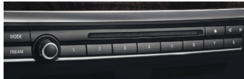
■ Memory buttons provide access to the most frequently used functions of the iDrive system. The eight convenient buttons allow the driver and front passenger to store and then easily access any functions of the Navigation system; the audio system – including specific radio stations or CD tracks; and the Bluetooth enabled mobile phone (if so equipped).
