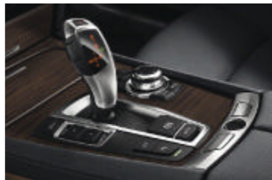
■ Automatic transmission provides extremely fast synchronized shifting. Gears are always changed electronically, whether performed in Automatic shift mode or Manual shift mode. The 760Li and ActiveHybrid 7 models offer eight speeds; all other models provide six speeds.
