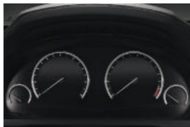
■ Black Panel Display shows the instrument cluster as a matte black surface when the ignition is switched off. Only the chrome rings of the circular instruments (open at the bottom) are visible in 3-D. When the doors are opened, the chrome rings join at the bottom and the analog dials and displays are shown. Then, when the ignition is switched on, the graphics display showing the trip computer and Check Control information light up.
