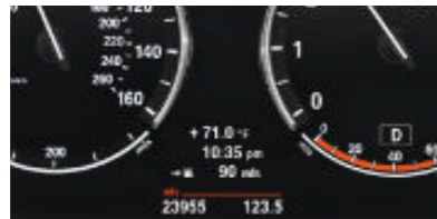
As soon as you brake or lift your foot off the throttle, Brake Energy Regeneration converts the braking energy released by the vehicle into electric power, and feeds it into the battery. The charge process is displayed by a symbol in the tachometer.
