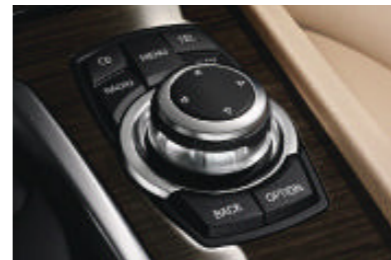
■ iDrive Controller is the central command element for the iDrive system and can be rotated, pushed and tilted to operate various functions via the Control Display. Additionally, four frequently selected menus – CD, radio, Navigation system and telephone – can be called up using direct menu-control buttons.
