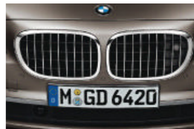
□ When equipped with the optional Night Vision with Pedestrian Detection system, the twin-kidney grille is slightly modified. Using nine vertical slats instead of the standard 13 provides an unobstructed view for the infrared camera's lens.
