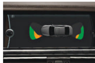
■ Park Distance Control (PDC) uses sensors located in the front and rear bumpers to facilitate parking and maneuvering in tight spaces. The driver is kept informed with an audible warning and also a graphic in the iDrive Control Display, showing the distance from the car to an obstacle.
