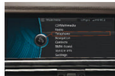
■ Control Display shows the functions supported by the iDrive Controller, such as the Navigation system, vehicle settings and radio. The high-resolution 10.2-inch color monitor is located next to the instrument cluster, at an ideal viewing height and distance.
