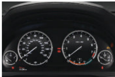
■ Dashboard with four analog instruments shows speed, rpm, fuel level and engine oil temperature above a high-resolution, wide-format Info Display. Also shown, as a graphic display, are the current fuel economy and range, as well as trip computer functions, an odometer and a daily trip recorder.
