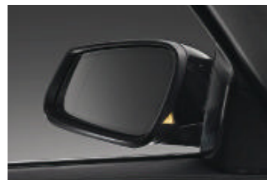
■/□ Active Blind Spot Detection warns if a vehicle is in your blind spot, or if a vehicle is approaching at high speed in the passing lane. This feature is activated when you use the turn-signal indicator before changing lanes.
