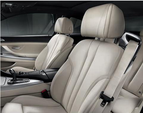
20-way power Multi-contour front seats conform to your body to provide optimum support and exceptional comfort over long distances. In addition to horizontal, vertical and angled adjustments, Multi-contour seats include an articulated upper backrest, comfort headrest (two-way power, two-way manual "relax headrest"), and four-way power-adjustable lumbar support. Both driver's and front-passenger's seats include memory function. Active front seats (not shown) imperceptibly raise and lower the left and right halves of the seating surface. This movement keeps the spine in motion, exercising various support muscles to help reduce fatigue on longer trips. Ventilated front seats (not shown) gently blow warm or cool air through the micro-perforations in the leather to keep driver and front passenger comfortably dry in hot weather, and warm in colder weather.
