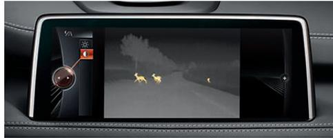
**BMW Night Vision with Pedestrian Detection** can scan up to 900 feet ahead using an infrared camera in the front bumper.<sup>1</sup> It can detect people and animals, as well as the direction of their movement, up to approximately 300 feet away, and displays their presence on the iDrive screen and Head-up Display. The system gives a visual warning as soon as pedestrians or animals move toward the road, alerting you to potential dangers significantly earlier, so you can react more quickly.
