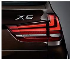
**Taillight cluster** with taillight, brakelights and turn-signal indicators incorporate LED technology for greater visibility. **Adaptive Brakelights** warn following vehicles by increasing in brightness when the intensity of your braking action is increased.
