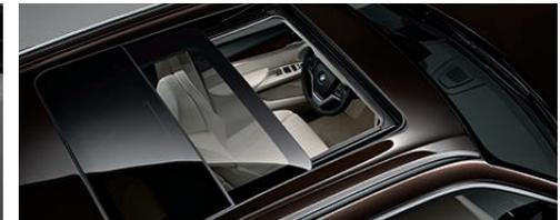
**Panoramic moonroof** is designed with generous dimensions to offer a stunning view, day or night. Easy-to-use features include a power slide and lift control, a comfort opening/closing function, a speed-sensitive wind deflector, and a power sunshade to shield passengers from excessive glare and heat. Both glass panels tilt up electronically at the touch of a button; the front panel also features a sliding function.
