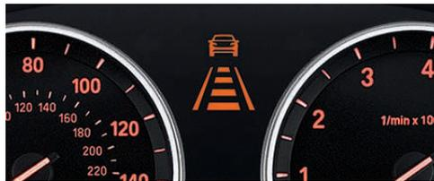
**Active Cruise Control with Stop & Go<sup>2</sup>** lets you preset desired speed and following distance. When it recognizes slower vehicles ahead, it reduces your speed to maintain the preset distance, and can even bring you to a complete stop if traffic calls for it. Active Cruise Control also includes the Active Driving Assistant features.
