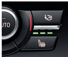
**Heated front seats** are a welcome feature in cooler weather. At the touch of a button, driver and front passenger can individually select from three heat settings.
