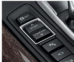
**Driving Dynamics Control including ECO PRO mode.** At the push of a button you can switch from the standard engine and transmission settings of COMFORT mode to the extra-efficient ECO PRO mode. Or select SPORT mode for an even more dynamic driving experience.
