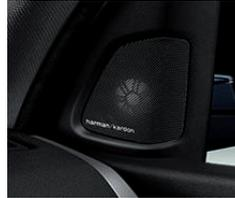
**Harman Kardon® Surround Sound system** is a 16-speaker system with 600-watt digital amplifier and Dirac signal processing that outputs reproduction of the surround information contained in the stereo signal in a nine-channel format, as well as 5.1 surround sound from a DVD source.
