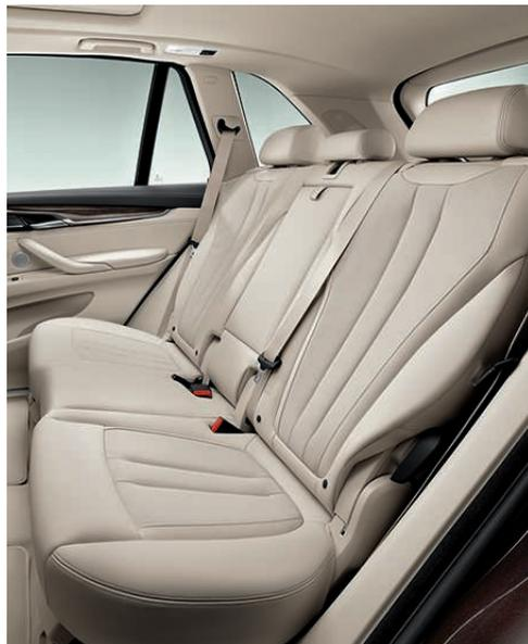
**Rear comfort seats** are specially upholstered for outstanding comfort. Both seats can be individually adjusted in numerous ways. The two outer seatbacks can recline 10 degrees in six stages. In a 60/40 split, they can also be moved 3.1 inches fore and aft, providing greater legroom or increasing the cargo space, as needed.
