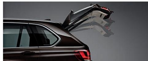
**Tailgate** opens in two sections. Lower the bottom section to create a platform that holds up to 550 lbs. The top section can be raised separately for quick removal of small items.
