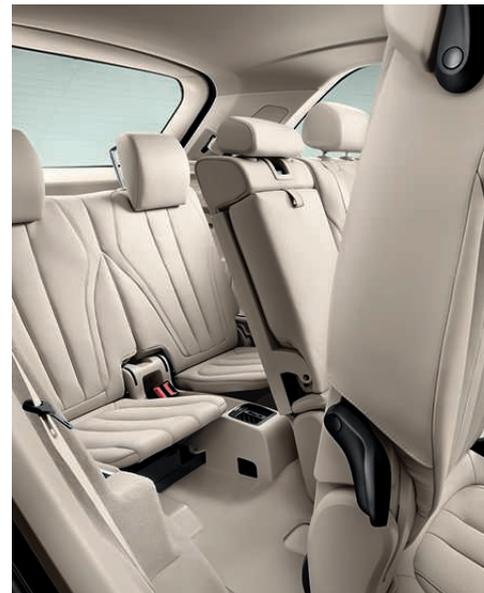
**Third-row seating** allows greater flexibility in transporting up to seven people. In addition to the two fold-down seats with inertia-reel safety belts, a center console includes two cupholders, and there is heating for the third-row footwells. The second row of seats can be folded down using the Easy Entry Function; there is also a grip plate by the C-pillar. When not in use, each third-row seat can be lowered individually into the floor for increased cargo space.
