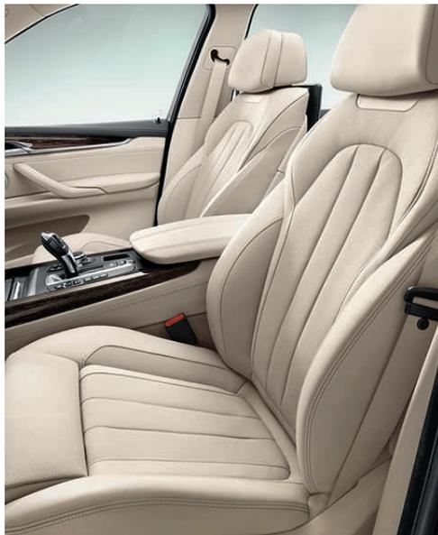
**Multi-contour seats** for driver and front passenger can be adjusted in various ways to provide personalized support and comfort. The top part of the backrest, the backrest width, thigh support and headrest height can be individually adjusted. Both front seats also feature Active Head Restraints, lumbar support and a memory function.
