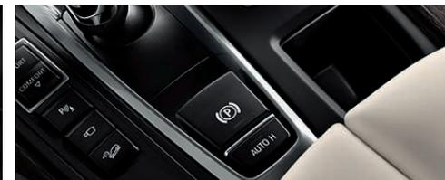
**Electromechanical parking brake with Automatic Hold** is activated via a button in the center console. This feature helps prevent the vehicle from rolling forwards or backwards when at a standstill, and keeps the vehicle stationary whenever it comes to a stop, such as in slow-moving traffic. The brake is released when you step on the accelerator.
