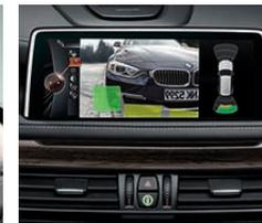
**Rear-view Camera** shows on the Control Display the area behind your vehicle. Guidelines indicate if your vehicle can fit in a parking space, and display parking turn angles. The Rear-view Camera is activated by engaging reverse gear.
