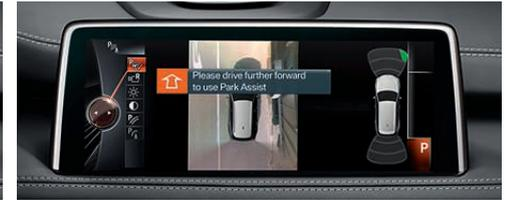
**BMW Parking Assistant** makes parallel parking a breeze. Suitable parking spaces can be shown and selected via the Control Display. Hold down the button and the system actively takes over parking, selecting the right gear, steering, accelerating and braking, as needed.
