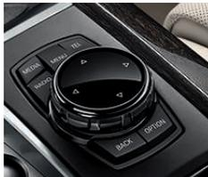
**Ceramic controls** present a deep black glazed finish to various controls, such as the iDrive Controller bezel, front and rear ventilation controls, and audio controls. The black ceramic provides a rich, custom look and unique feel to the interior.
