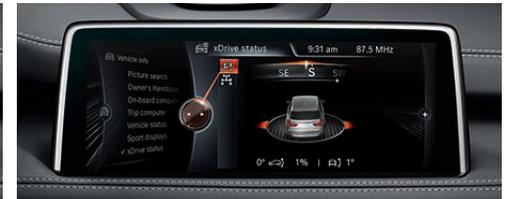
**iDrive Status** shows, in the Control Display, 3-D real-time information about the vehicle's body roll and pitch. A compass display is also shown in the instrument cluster.
