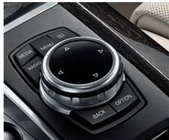
**iDrive touchpad Controller** allows intuitive, convenient operation of the iDrive system. Using the Controller-integrated touchpad, you can enter destination addresses for the Navigation system by using your own handwriting, while the input is conveniently shown in the Control Display.
