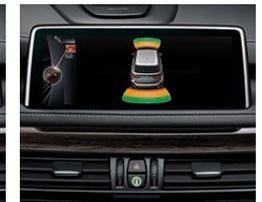
**Automatic Park Distance Control** engages when the system detects a parking maneuver. This helps you judge distance to other vehicles and unseen objects when parking. The warning beeps come faster as the bumper approaches the object, turning into a constant tone at less than 12 inches.
