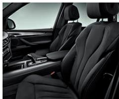
**10-way power front sport seats** with driver's-seat memory system include power-adjustable seat height, seat angle, backrest angle and lumbar support, and two-way manual thigh support. Contoured side bolsters cradle you comfortably over long distances, while holding you firmly in place during sporty driving maneuvers.
