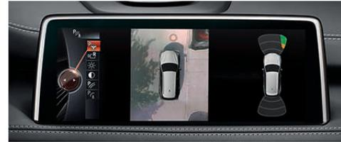
**Surround View** makes it easier to park and maneuver in tight spaces. The area behind and on either side of the vehicle is shown on the Control Display from a bird's-eye perspective (Top View). This is combined with Side View, which assists you when approaching areas with limited visibility (such as when exiting driveways or parking garages).
