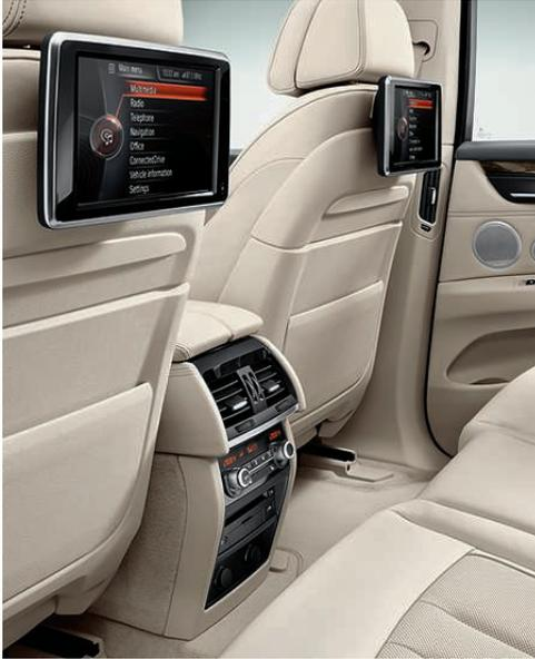
**Rear-seat entertainment** includes two freestanding, tablet-style 9.2-inch color screens integrated into the back of the front seats. The system includes a remote Controller and headphone jacks.
