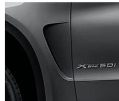
**Air Breathers**, located in the front wheel arches, channels the airflow at the front wheels. This decreases air turbulence at the front wheels, thereby reducing fuel consumption.
