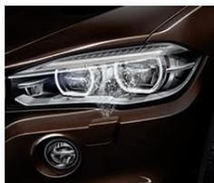
The **headlight washing system** maximizes illumination of the road ahead in all weather. When the windshield washer function is activated, headlights are also automatically cleaned.
