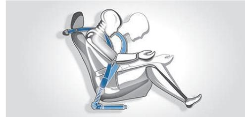
**BMW restraint system** for driver and front passenger combines three-point safety belts, automatic safety-belt pretensioners, and seat bolsters that help prevent occupants from sliding forward. Active Head Restraints in the front seats reduce the risk of whiplash or neck/head/spine injury. When sensors detect a rear-end collision, the headrests automatically and rapidly pivot forward, supporting the occupant's heads.
