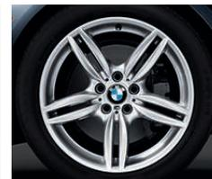
**Double Spoke (Style 351M)** light alloy wheels. With run-flat¹ performance tires²-³: 19 x 8.5 front, 19 x 9.0 rear and 245/40 front, 275/35 rear tires. (Includes increased top-speed limiter.) With run-flat¹ all-season tires²: 19 x 8.5 and 245/40 tires.
