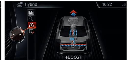
**Boost function.** When required, energy from the high-performance lithium-ion battery is used to enable a short-term 55-horsepower boost. A benefit of this technology is strong and immediate power delivery.
