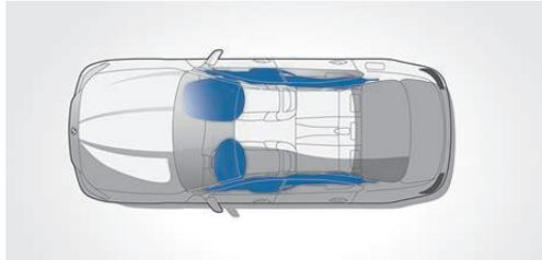
**Airbags.** In the event of a collision, BMW's supplemental restraint system (SRS) determines which airbag(s) to deploy for optimal protection. When a safety belt is used, airbags deploy only at a higher crash severity; the force of the deployment depends upon the severity of the impact. Driver and front passenger airbags, the Curtain System with head airbags as well as front seatback-integrated side airbags provide effective protection for you and your passengers in the event of a collision.
