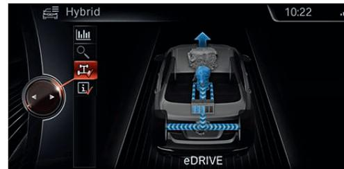
**All-electric driving.** The output of the electric motor allows all-electric driving over longer distances. Using Driving Dynamics Control to activate the ECO PRO mode, the transmission uncouples the engine and shuts it off when you take your foot off the accelerator. This feature enables the BMW ActiveHybrid 5 to "sail" downhill almost silently at speeds of up to 100 mph. When the ECO PRO mode is deactivated, it is possible to sail at speeds of up to 50 mph.
