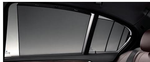
**Power rear sunshade** can be extended with the touch of a button to protect the cabin from the sun's rays in warm weather, or retracted to allow the sun to help warm the interior in colder weather. **Manual rear side sunshades** keep the sun's heat and glare away from the rear cabin while maintaining your privacy. When not in use, they conveniently disappear into the side doors.
