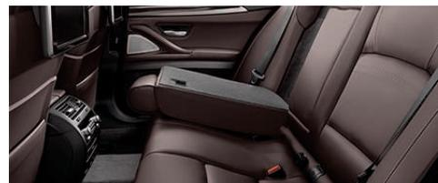
**Through-loading system** includes a 60/40 split-folding rear seat for greater flexibility in seating and cargo combinations. The center armrest includes an integrated storage compartment with two cupholders; a matching ski and snowboard bag is available from Original BMW Accessories.
