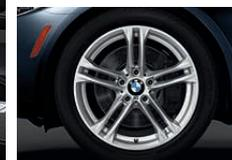
**Double Spoke (Style 613M)** light alloy wheels. With **run-flat<sup>1</sup> performance tires<sup>2,3</sup>**: 18 x 8.0 front, 18 x 9.0 rear and 245/45 front, 275/40 rear tires. (Includes increased top-speed limiter.) With **run-flat<sup>1</sup> all-season tires<sup>2</sup>**: 18 x 8.0 and 245/45 tires.
