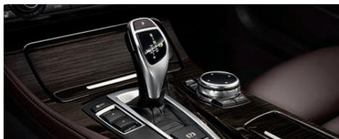
**8-speed Sport Automatic transmission** with Adaptive Transmission Control (ATC) provides extremely fast synchronized shifting in either the Sport or Manual shift mode; racing-inspired steering wheel-mounted paddles are also included. New in the 550i and 550i xDrive: Launch Control, for optimized traction and maximum dynamics when accelerating from a standstill.
