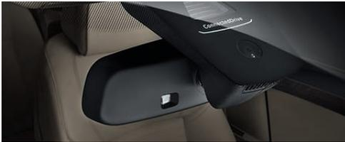
**Rain sensor** monitors the intensity of the rain and automatically regulates the windshield wiper interval. It also automatically turns on the low beams when needed.
