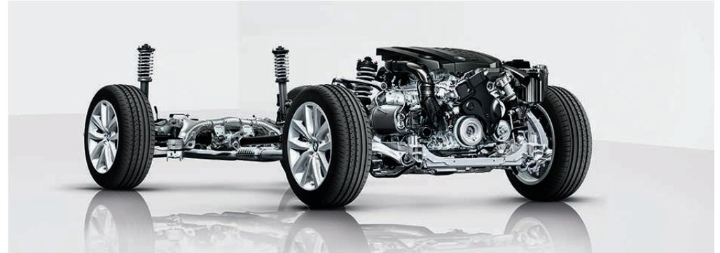
**Integral Active Steering**, in rear-wheel-drive vehicles, delivers more direct response with a small turn of the steering wheel at speeds of up to 30 mph. This feature also steers the rear wheels up to 2.5 degrees in the opposite direction, giving the effect of a shortened wheelbase for enhanced maneuverability. When changing lanes at speeds over 50 mph, both front and rear wheels turn in the same direction, giving the feel of an extended wheelbase.
