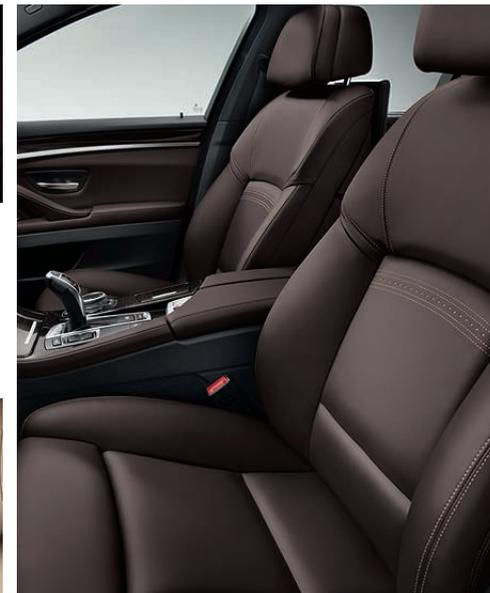
**20-way power Multi-contour front seats** conform to your body to provide optimum support and comfort over long distances. In addition to horizontal, vertical and angled adjustments, Multi-contour seats include an articulated upper backrest, Comfort headrest (two-way power, two-way manual "relax headrest"), power-adjustable side bolsters and four-way power lumbar support. Both driver's and front-passenger's seats include memory function.
