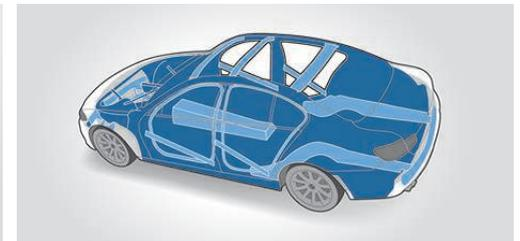
**Body stiffness.** The intelligent use of high-strength multi-phase steel and aluminum provides a high degree of body stiffness and crash resistance. Components, such as the A-pillars and windshield frame, include special reinforcements to provide optimum occupant protection.
