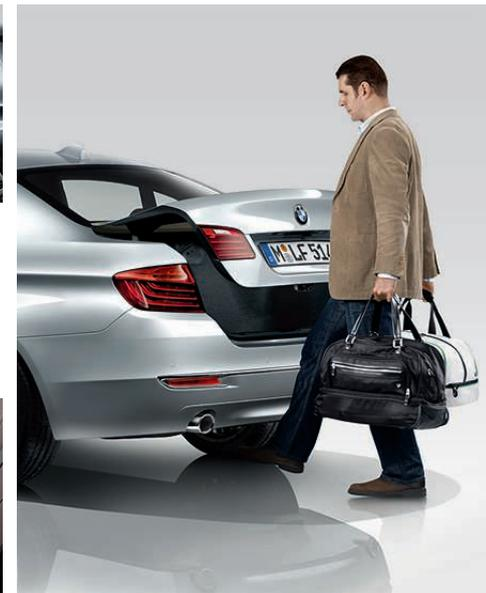
**Comfort access system** offers convenient keyless access to the driver's door, front passenger door and trunk when you carry the remote key in a pocket or purse, simply by touching the door handle. The hands-free trunk-lid opening function automatically unlocks and opens the trunk when you move your foot under the center of the rear bumper. Repeat the motion to close the trunk.
