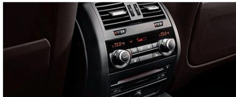
**4-zone automatic air conditioning** builds on the 2-zone system with air vents in the B-pillar and at the rear of the center console, to ensure virtually draftless ventilation for rear-seat passengers. Additionally, the temperature in both the left and right rear cabin can be tailored via two control dials with displays.
