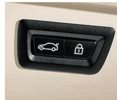
**Automatic trunk-lid operation** makes opening and closing easy. All it takes is a simple press of a button on the A-pillar on the driver's side or on the vehicle key. A button in the trunk lid also makes closing easy.
