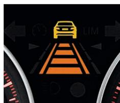
**Active Cruise Control with Stop & Go** lets you preset desired speed and following distance. When it recognizes slower vehicles ahead, it reduces your speed to maintain the preset distance, and can even bring you to a complete stop if traffic calls for it. Active Cruise Control also includes the Active Driving Assistant features.
