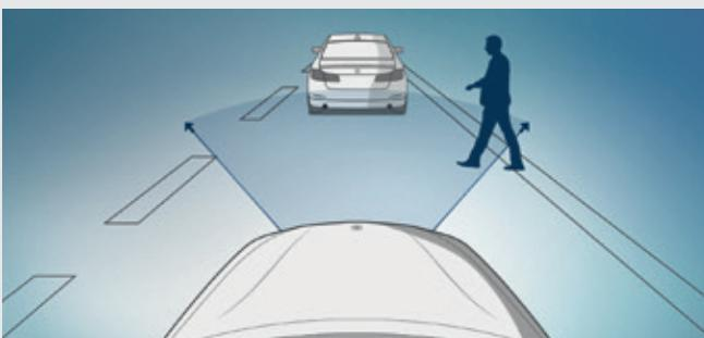
■ **Person warning with city braking function** actively assists the driver with the prevention of collisions involving pedestrians. It is active at speeds of up to 35mph and preconditions the brakes for increased responsiveness. In the event of an emergency, the system prevents a collision or ensures that the collision speed is considerably reduced.<sup>2</sup>
