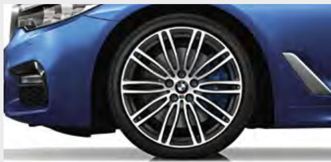
■ 19" M light alloy Double-spoke style 664 M wheels, front 8J x 19 with 245/40 R19 tyres and rear 9J x 19 with 275/35 R19 tyres.
