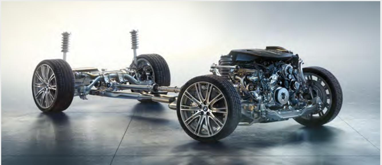
**Integral Active Steering** combines support that varies based on the steering angle on the front axle, and rear wheels that also contribute to steering. At lower speeds, it offers greater manoeuvrability and agility by turning the rear wheels opposite the front wheels. Beginning around 37mph, the rear wheels turn parallel to the front wheels, to increase stability and comfort.<sup>1</sup>
