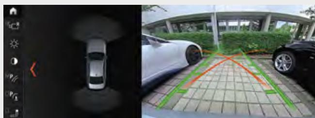
□ The reversing assist camera enables improved orientation when reversing at speeds below 10mph, for example when parking. It shows the area behind the car on the Control Display. Interactive track lines for measuring distance and turning circles assist the driver when manoeuvring, obstacles are marked in colour.
