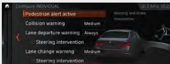
□ Driving Assistant Plus offers automatic driving with greater comfort and security in monotonous and dangerous situations. These can include on the one hand traffic jams, slow-moving traffic or long journeys through the city, on country roads or motorways and on the other hand navigating junctions and hazardous lane changes. The vehicle takes action when the driver either cannot or will not.
