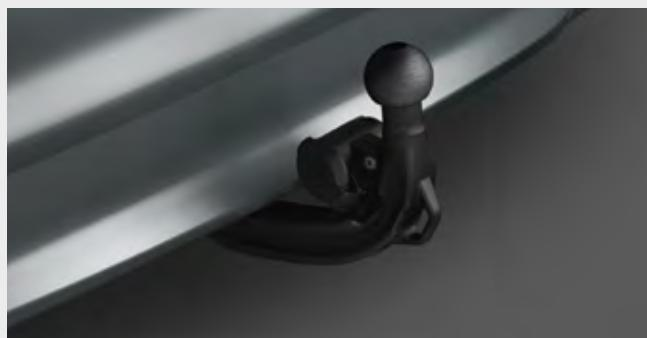
□ The Towbar with electrically adjustable tow ball is approved for heavy loads of up to 2,000kg. In order to stabilise things, trailer stability control automatically brakes the pulling vehicle if the trailer begins to swing. The electronically adjustable tow ball is not visible when stowed under the rear apron.
