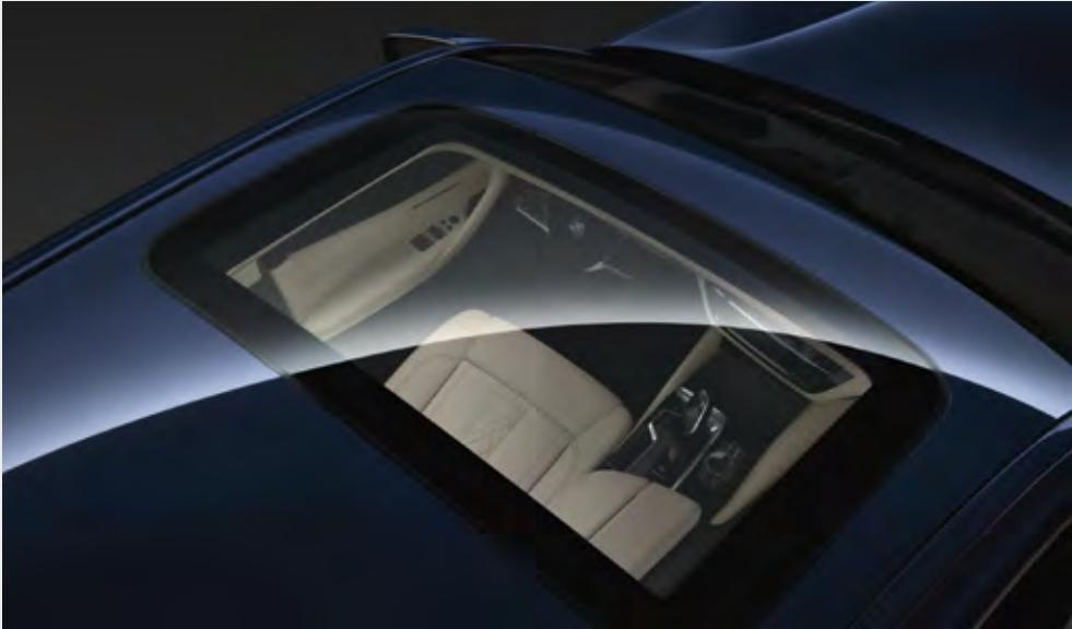
□ The electric glass sunroof with slide and lift function, including an electric sliding interior roof, anti-trap protection, as well as comfort opening and closing, allows the airflow to be individually regulated to create a pleasant interior climate. The integrated wind deflector prevents draughts from developing in the interior and ensures a lower level of wind noise.
