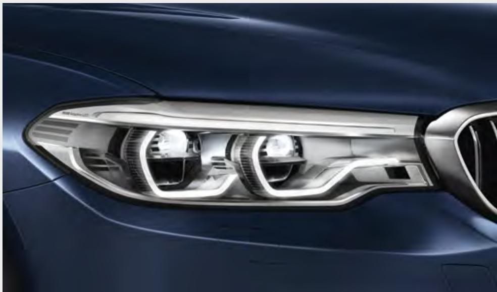
□ The BMW Icon Adaptive LED Headlights include BMW Selective Beam, cornering lights and adaptive headlights. The light colour is similar to daylight and provides an ideal, even illumination of the road to improve visibility and make driving in the dark less tiring. The iconic light design with four light elements makes the vehicle recognisable as a BMW even at night.
