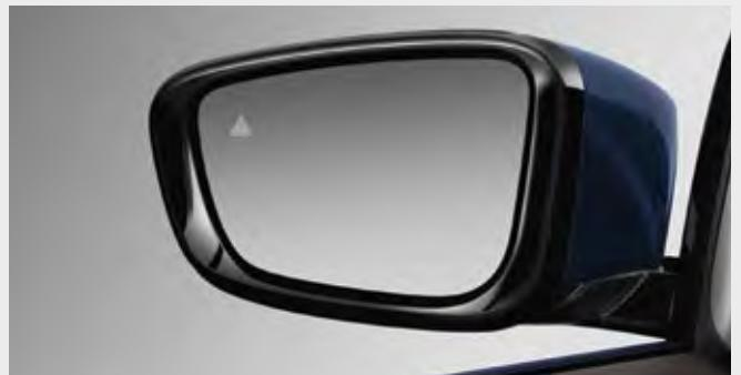
□ If the indicator is on, the radar-based Lane Change Warning<sup>2</sup> warns the driver of approaching vehicles in the blind spot as well as vehicles in the neighbouring lane. The system functions beginning at speeds of 6mph, and in dangerous situations, it causes the steering wheel to vibrate and the triangle symbol in the exterior mirror to blink.
