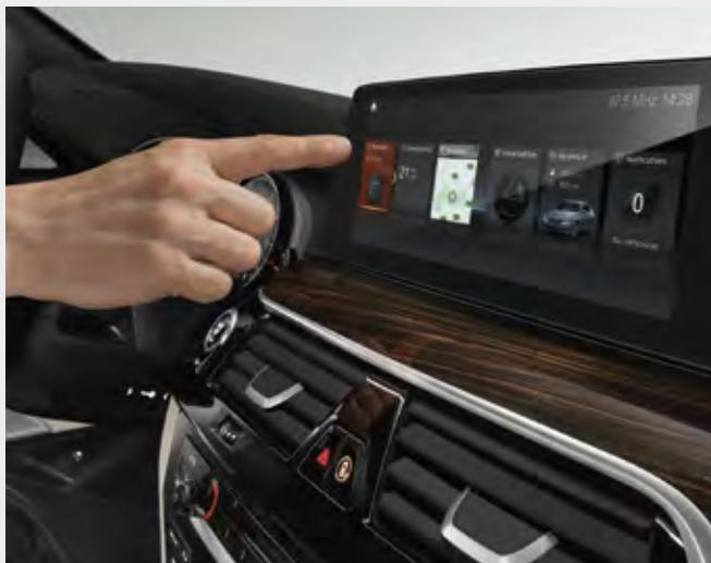
□ With BMW Gesture Control, certain functions can be operated by means of defined hand movements. For certain operations the system will for example recognise gestures such as 'swiping' or 'pointing' for accepting or rejecting an incoming call, or circular motions of the index finger to adjust volume.
