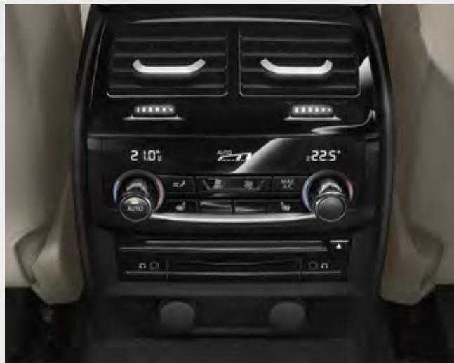
□ Automatic air conditioning with four-zone control comes with the equipment included in automatic air conditioning with two-zone control with extended features, along with two air vents in the B columns. Additionally, the rear passengers can individually adjust their own climate via a separate control element with display.
