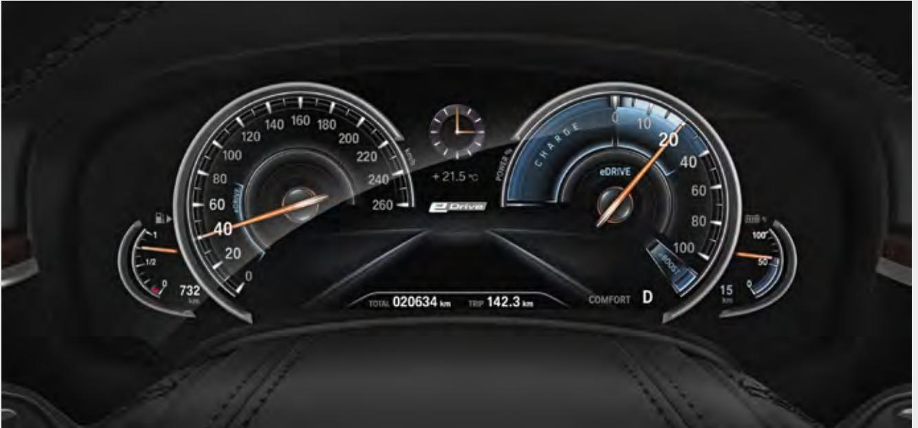
The instrument cluster includes dials that help the driver to make particularly efficient use of the electric drive with information such as battery charge level and drive status.
