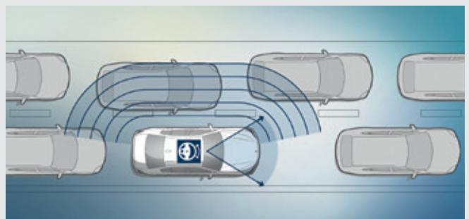
□ The **Lane Departure Warning** detects lane markings and alerts the driver before an unintentional lane change at speeds above around 45mph by means of vibrations in the steering wheel. The warning is not activated if the lane change is deliberate, that is, when the indicator has been activated.<sup>3</sup>
