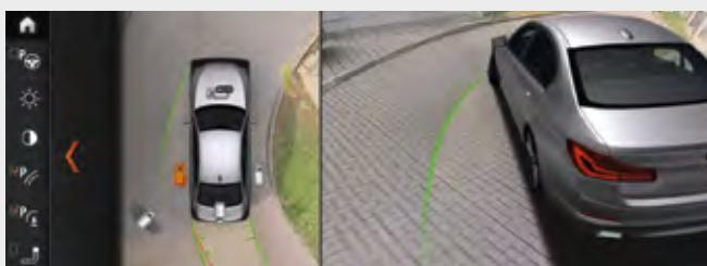
□ Parking Assistant Plus makes parking and manoeuvring the vehicle easier. It features Surround-view including Top-view, Remote 3D view, Panorama view, PDC and Park Assist with linear guidance, which parks the vehicle parallel or perpendicular to the lane completely automatically. The system works by measuring potential spaces while driving past at a low speed.
