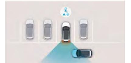
**Rear Cross Traffic Alert (RCTA):** When reversing out of a narrow parking space, the Rear Cross Traffic Collision Warning reduces the risk of a collision. Using 2 radar sensors at the rear, it warns you in case of any approaching cross traffic.
