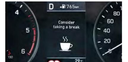
**Driver Attention Alert (DAA):** This available feature from SE Nav and above raises safety and convenience to an entirely new level by continuously monitoring and analysing driving patterns. When a pattern of fatigue or distraction is identified, DAA gets the driver's attention with an audible alert and pop-up message suggesting a break.
