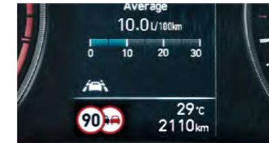
**Intelligent Speed Limit Warning (ISLW):** The Intelligent Speed Limit Warning uses the front camera and information from the navigation system to identify road speed signs and displays the speed limit and no-passing signs in real time. The information is displayed in both the navigation system display and the TFT cluster.
