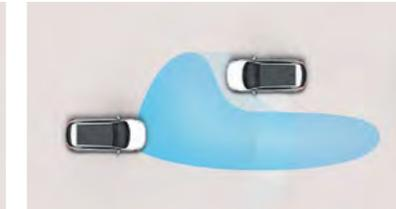
**Full LED Lighting Technology:** High Beam Assist (HBA) detects oncoming vehicles as well as vehicles in the same lane ahead at night, and changes from high beam to low beam as appropriate. The Static Cornering Light illuminates the front side area ahead when cornering, improving visibility at night.
