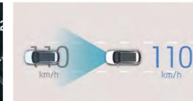
**Advanced Smart Cruise Control (ASCC) with Stop & Go function:** Using front radar sensors, Advanced Smart Cruise Control with Stop & Go function keeps a constant speed and distance from the vehicle ahead by automatically accelerating and braking. If traffic comes to a halt, the Stop & Go system applies the brake until the car comes to a standstill and accelerates to the desired speed as soon as the road is clear.
