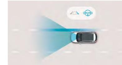
**Lane Keep Assist (LKA):** The standard LKA uses the front camera to monitor the lines of the road. In case of an unintended lane departure, it will warn the driver and can apply counter steering torque to guide the car back to the lane.
