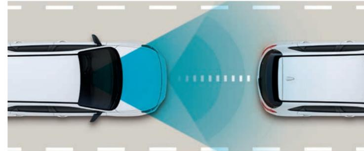
**Autonomous Emergency Braking (AEB):** Automatically applies partial or maximum braking force if a potential collision is detected.
