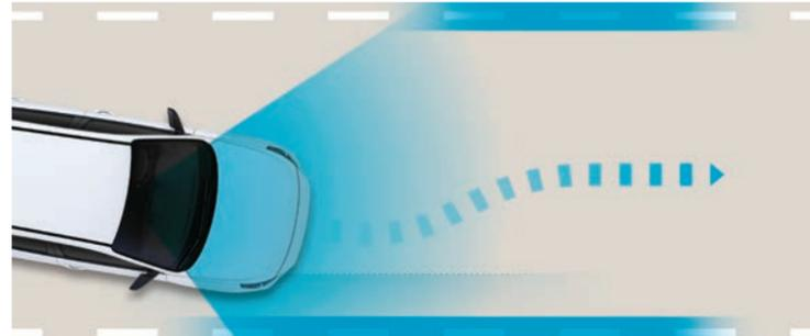
**Lane Keeping Assist (LKA):** At speeds over 37 mph the system alerts the driver about unsafe movements. In case of an unintended lane departure, it will warn the driver and can apply counter steering torque to guide the car back to a safe position.
