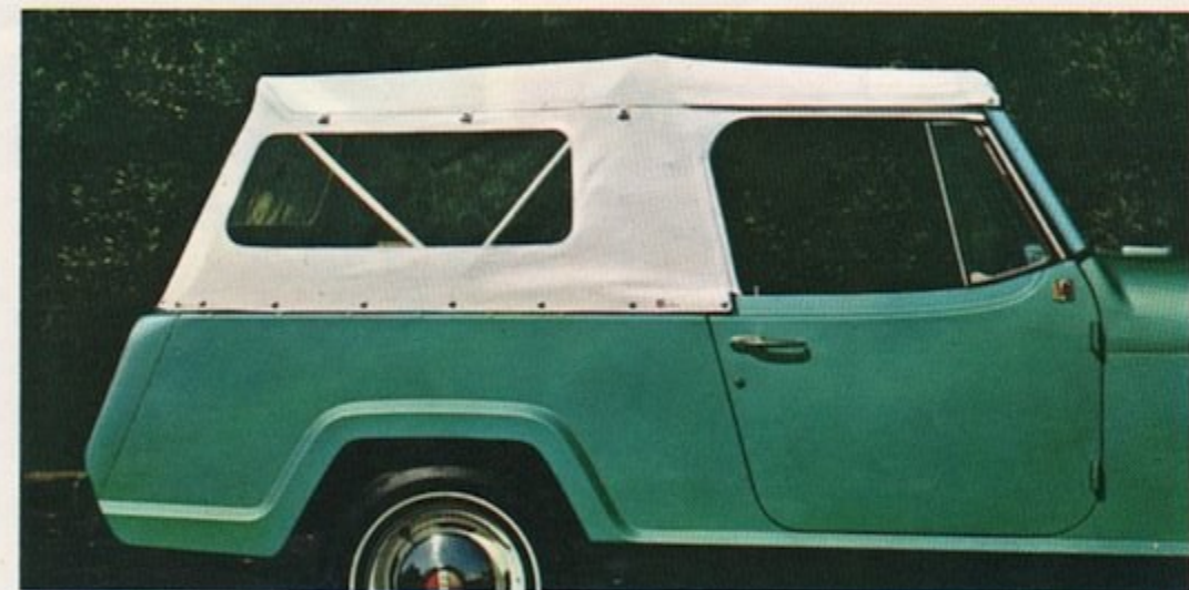
Soft top (station wagon style) with non-yellowing vinyl rear quarter and tailgate windows. Rear seat is also available.
