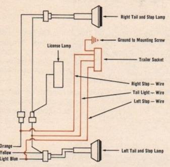
The diagram above indicates the wiring connections required to effect the simultaneous flashing of trailer brake lights and trailer directional signals. When this system is used, a variable load flasher — available from your 'Jeep' dealer — must be used. When your 'Jeep' vehicle is not used for towing, it is recommended that the original flasher be re-installed. If your vehicle is equipped with 4-way warning lights, it is not necessary to change the variable load flasher.
