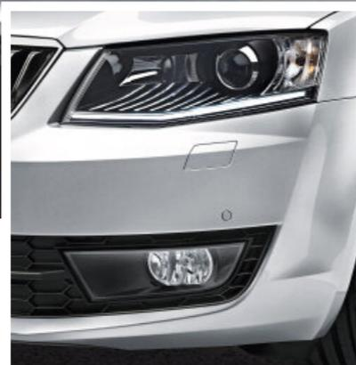
**Bi-Xenon lights.** The optimal illumination of the Bi-Xenon lights is enhanced by the AFS which changes the light setting depending of the car's speed and weather conditions. Bi-Xenon headlights provide 2.5 times the illumination of halogen headlights.
