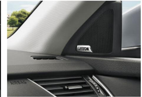
**Sound system.** For those who love their music, the standard 8 speaker sound system on Octavia can be upgraded to a Canton sound system which adds a central speaker to the dash and a subwoofer in the boot. Canton also adds a digital equaliser and sound level controls allowing spacial optimisation for all or individual occupants, vehicle noise cancellation and when added in combination with a 'Columbus' satellite navigation, the ability to play Dolby 5.1 surround sound.
