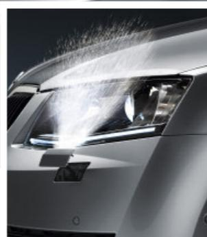
**Telescopic front headlight washers.** Standard on Elegance and vRS, optimise your front lights' range by keeping the front panels clean of dirt and debris.
