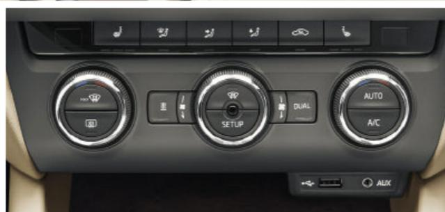
**Air conditioning.** Depending on trim, your Octavia will either be equipped with air conditioning or dual-zone air conditioning with humidity control. Dual-zone allows the driver and front seat passenger to set different temperatures for optimal comfort whilst the humidity sensor directs the airflow as required to keep the windscreen fog free.
