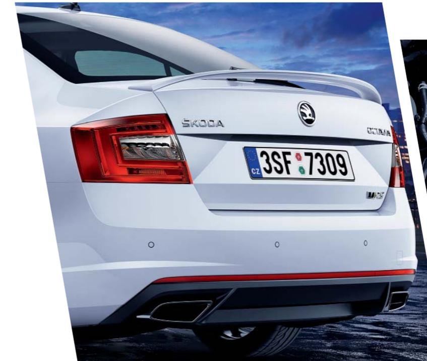
The exhaust pipe end pieces in glossy black finish have been specially tuned to produce the engine's characteristic sporty sound.
