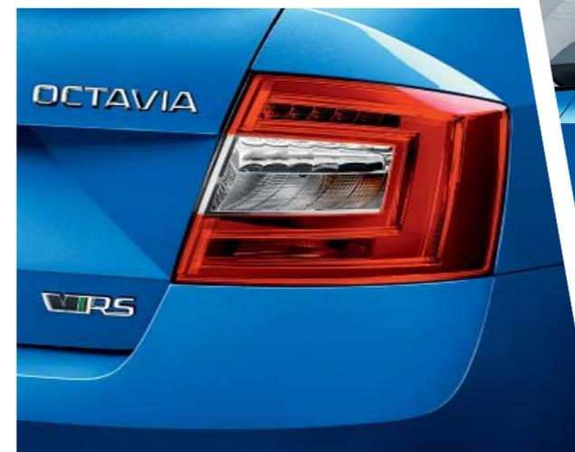
The rear lights, illumination of which creates a double C letter, are equipped with energy efficient LED diodes. The 5th door bears the OCTAVIA model name badge as well as the RS logo.
