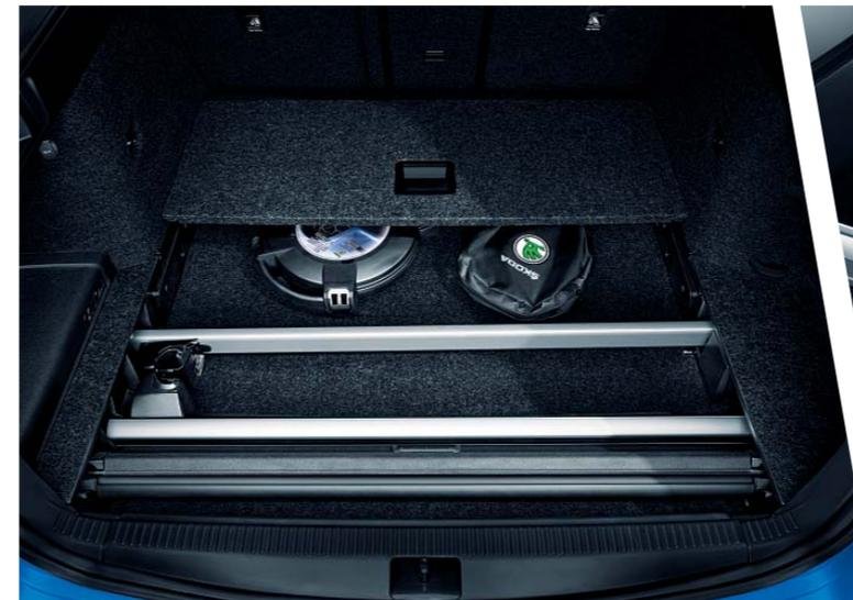
The double floor provides you with a hidden storage compartment. Simultaneously, it facilitates handling luggage by bringing the floor of the luggage compartment closer to the loading edge.
