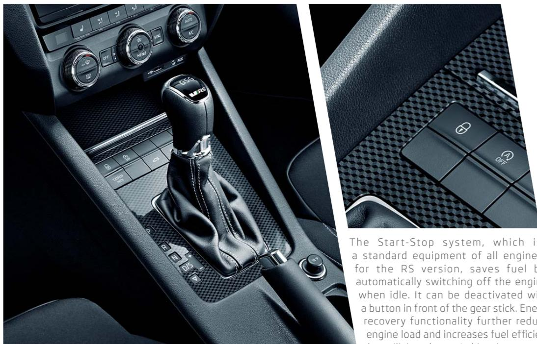
The Start-Stop system, which is a standard equipment of all engines for the RS version, saves fuel by automatically switching off the engine when idle. It can be deactivated with a button in front of the gear stick. Energy recovery functionality further reduces engine load and increases fuel efficiency by utilising the car's kinetic energy for battery recharging.
