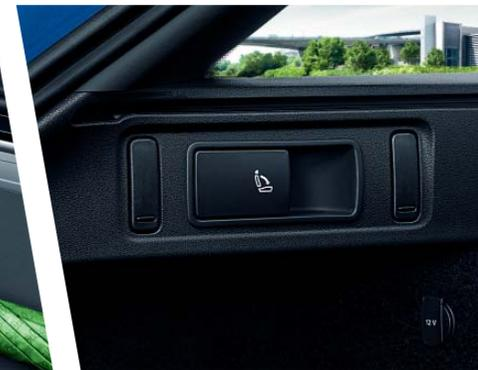
The rear seats can be folded using a remote release button located in the luggage compartment, which will make loading the car even more effortless.
