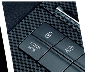
The Performance Mode Select includes the Performance Sound Generator function allowing the sound of the engine in the cabin to be set to the normal, eco or sport mode.
