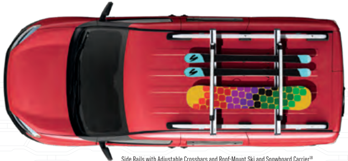
Side Rails with Adjustable Crossbars and Roof-Mount Ski and Snowboard Carrier 18
