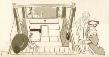
The interior fittings of the landaulet include arm rests, vanity cases, dictaphone, capacious door pockets and forward folding, disappearing auxiliary seats. The window regulators are trim in appearance and convenient in operation.
