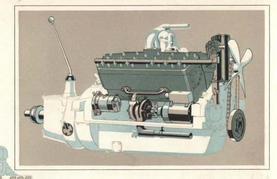
Cylinder heads are removable. In manufacturing, this feature admits of perfect machining, which in turn insures uniform compression. An improved channeling of the gas passages provides even more efficient distribution of the fuel to the combustion chambers.
