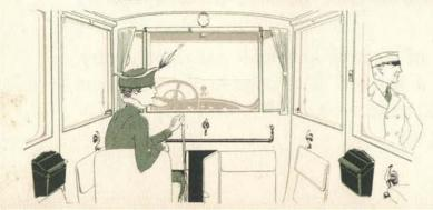
The auxiliary seats, folded, fit neatly into the back of the front seat; in position for use, they are in harmony with the beauty of the interior, ample and comfortable. Between them is a parcel compartment that may be locked. The 3-25 BROUGHAM
