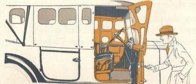
Metal door standards hold the curtains in upright position and allow the curtain to swing open with the door. The outside handles are a great convenience in stormy weather.
