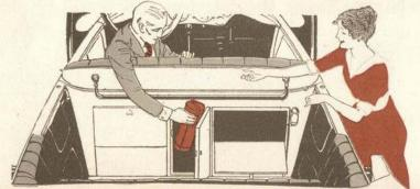
In the phaeton, the back of the front seat contains two compartments with doors that hinge about half way and swing from the top, and a center compartment that may be securely locked. They are just right for the things a small party wants to take along on a short trip.
