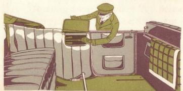
Umbrellas and walking sticks may be carried conveniently in a Packard touring car. On the opposite side is a special compartment for carrying the door curtain standards.
