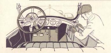
Controls and gauges are grouped with definite relation to the driver's convenience. All dials are plainly lettered and fall in the direct line of vision. Your hand reaches straight to the switches on the cowl board and your eyes keep to the road ahead. The 3-25 SALON TOURING
