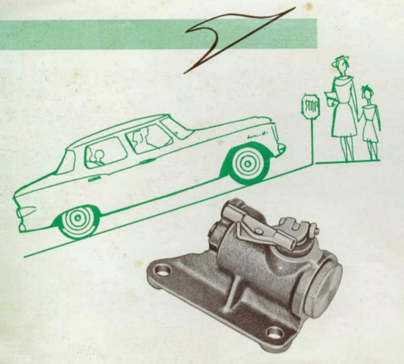
AUTOMATIC HILL HOLDER. One of many Studebaker engineering "firsts". Prevents rolling backwards on upgrades after braking to a stop. Simply keep the clutch pedal depressed and your right foot remains free to operate the accelerator on the take-off. For all models equipped with standard and overdrive transmissions.
