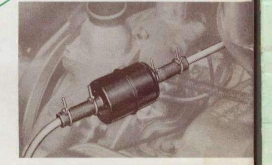
AC-2987 IN-LINE GASOLINE FILTER KIT. Assures smooth top performance and economy by removing dirt, moisture and foreign elements from the gasoline. Eliminates pressure surges and carburetor flooding caused by dirt holding open the needle valve.
