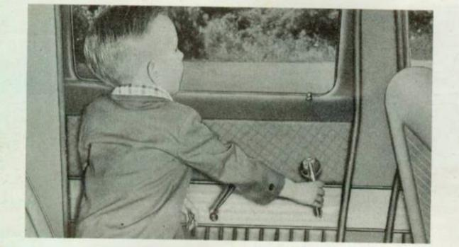
SP-50079 CHILD-GUARD REAR DOOR SAFETY LOCKS. Peace of mind for the driver . . . and protection for the children in the rear. Locks replace regular rear door lock buttons. When depressed in the locked position, they remain locked until opened by inserting key.
