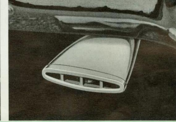
AC-2840 EXHAUST DEFLECTOR, A handsome complement in easy-to-clean stainless steel designed for use on Hawk models and most cars. Protects the chrome surface of the bumper by deflecting corrosive and injurious gases away from the exposed surfaces.
