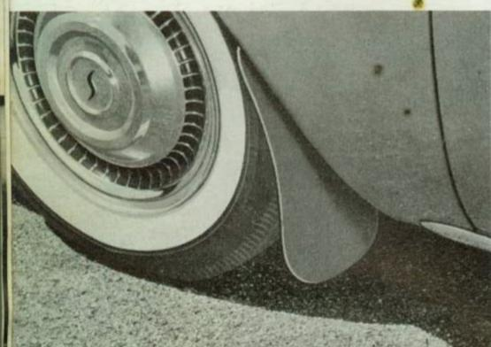
AC-2028 SPLASHGUARDS. Especially designed to deflect dirt, gravel and road oil thrown back by the front wheels and to protect the paint finish. Constructed of long lasting heavy-duty rubber reinforced with a steel insert at fastening points. Black only.
