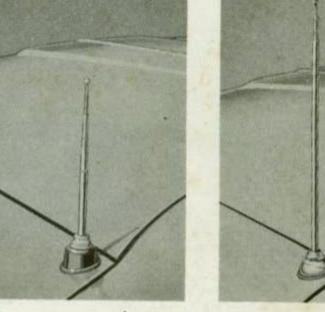
AC-2688 INTERNALLY CONTROLLED REEL TYPE ANTENNA. (Left) This popular front cowl mount reel type antenna has exclusive features engineered by Studebaker for top performance and ease of operation. It is controlled from inside the car by a knob which is located within easy reach of the driver.
