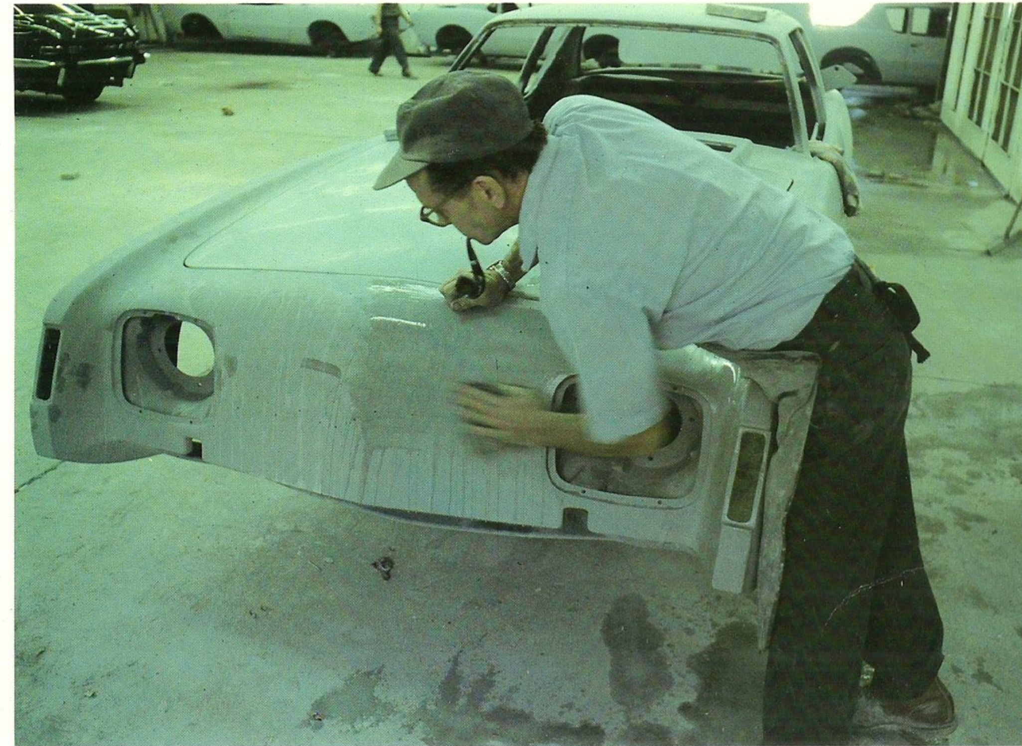
BELOW: Hand sanding of first coats of primer.
