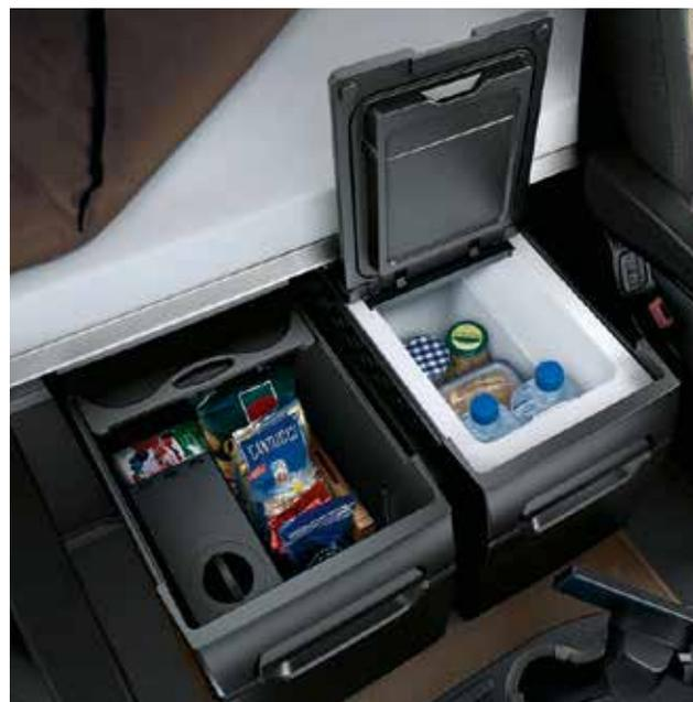
**Drawers under the bed.** The GigaSpace and BigSpace are equipped with two spacious drawers, one of which can optionally take the form of a refrigerator with a capacity of 36 l in which drinks bottles can be carried standing upright<sup>2)</sup>.
