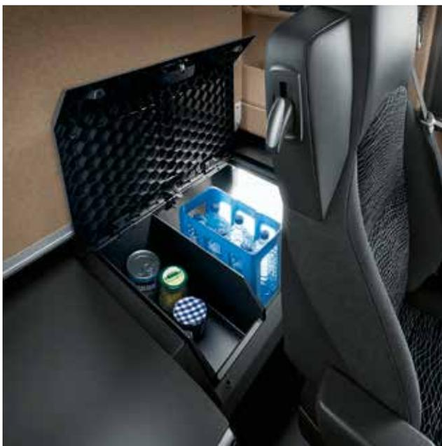
**Exterior stowage compartments.** With a capacity of up to 420 l, the two stowage compartments located under the bed in the L-cabs can be accessed from both the inside and outside and offer a huge amount of stowage space. Two adjustable stowage trays are optionally available to allow better use to be made of the space.
