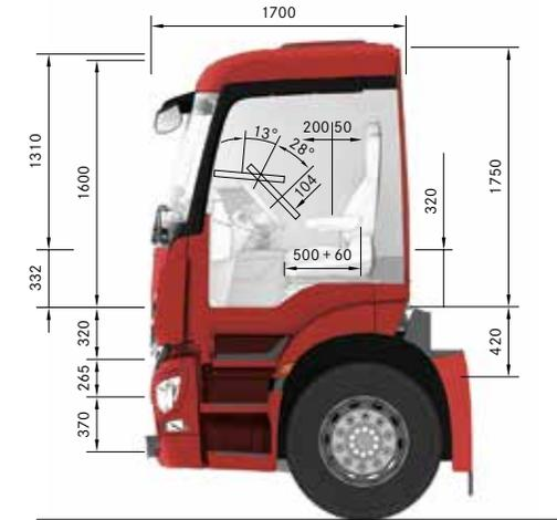
Engine tunnel: 320 mm
