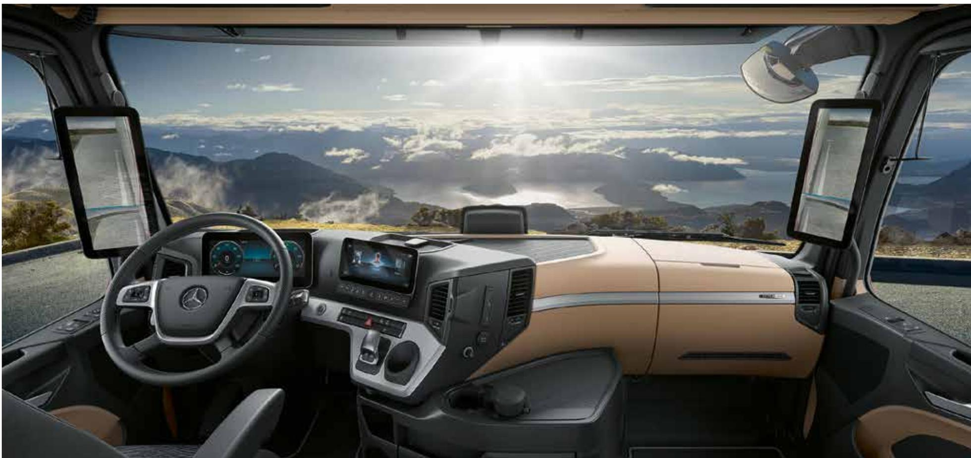
**Multimedia Cockpit<sup>1)</sup>**. The new Actros features the innovative Multimedia Cockpit for enhanced driving comfort, ergonomics and ease of operation. The new, state-of-the-art workplace comprises four screens in all. The primary colour display and the secondary Multi-Touch-Display, each with a screen diagonal of 10", can be operated via the new multifunction steering wheel with Touch Control Buttons.
