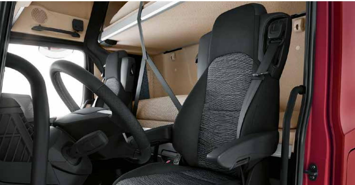
**Air-conditioned suspension seat.** The optionally available air-suspended, ventilated driver's suspension seat provides pleasant seating conditions and a high level of comfort. The integral armrests and the seat heating also contribute to this. The active ventilation system in the backrest and cushion of the climatized suspension seat reduces heat and moisture build-up. The numerous individual adjustment options make for optimal ergonomics.
