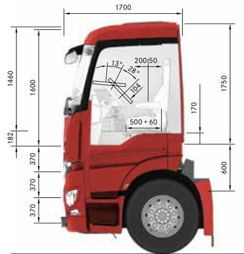
Engine tunnel: 170 mm
