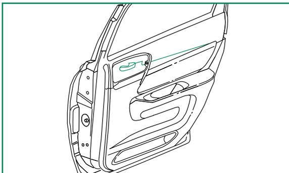
Inside rear door handles are disconnected. Rear doors can only be opened from the outside.
