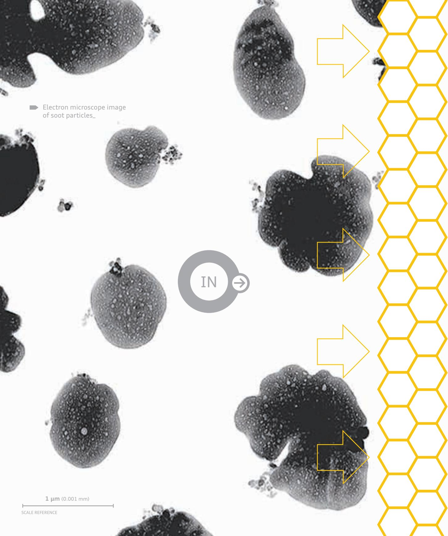
➔ Electron microscope image of soot particles\_
