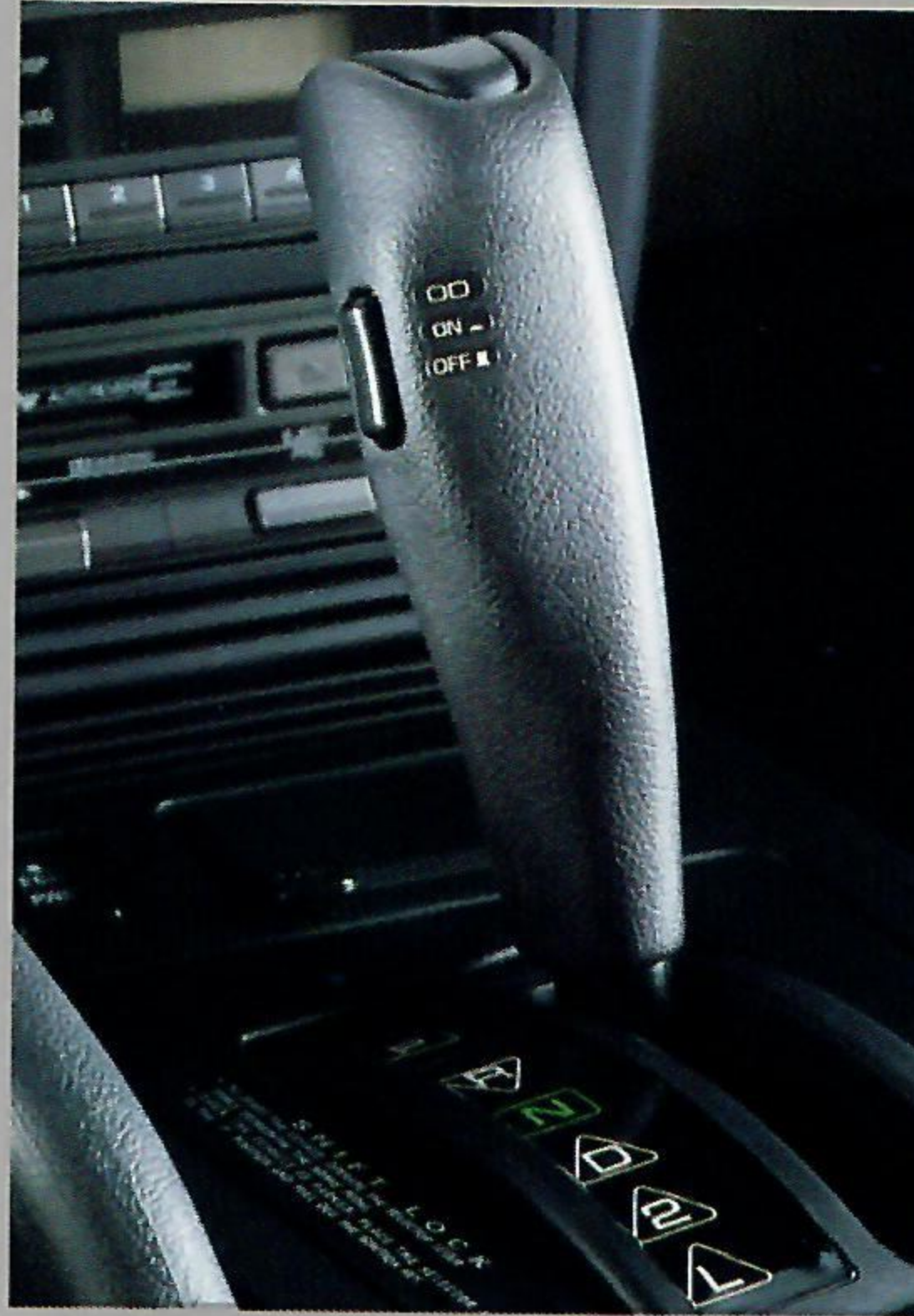
An optional 4-speed automatic overdrive transmission features a console-mounted Power/Economy switch and overdrive lockout button on the shifter.
