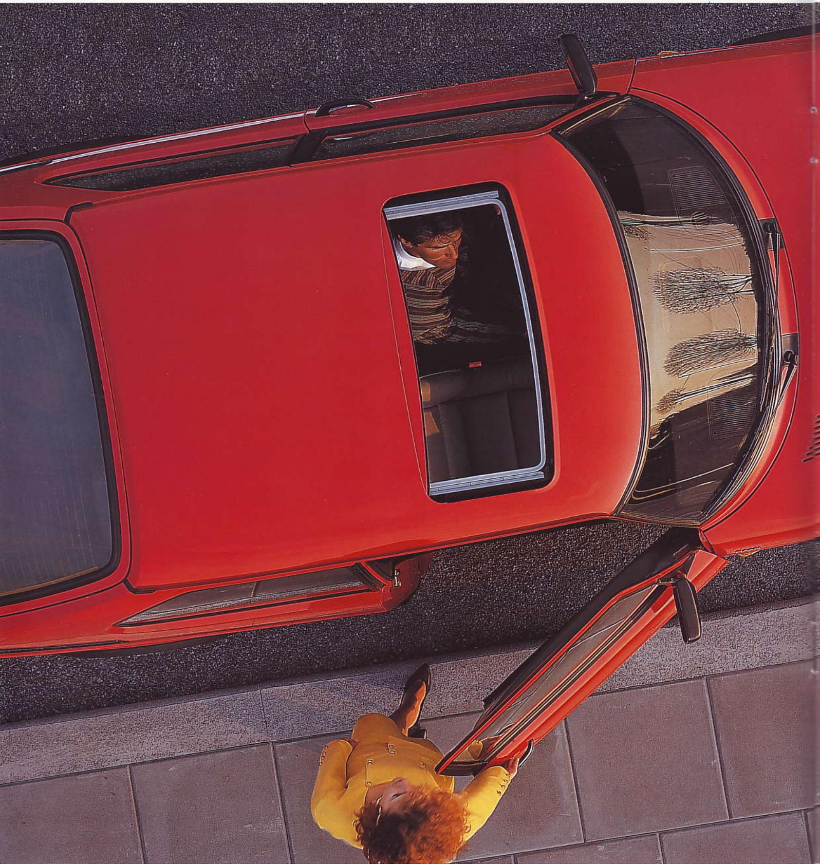
The deeply curved windshield improves aerodynamics, uses wind force to push rain, snow and dirt to the sides, and enhances safety by moving the glass farther forward from the front-seat occupants.
