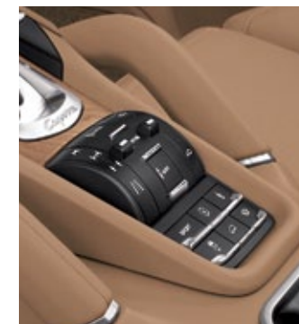
Main off-road control
