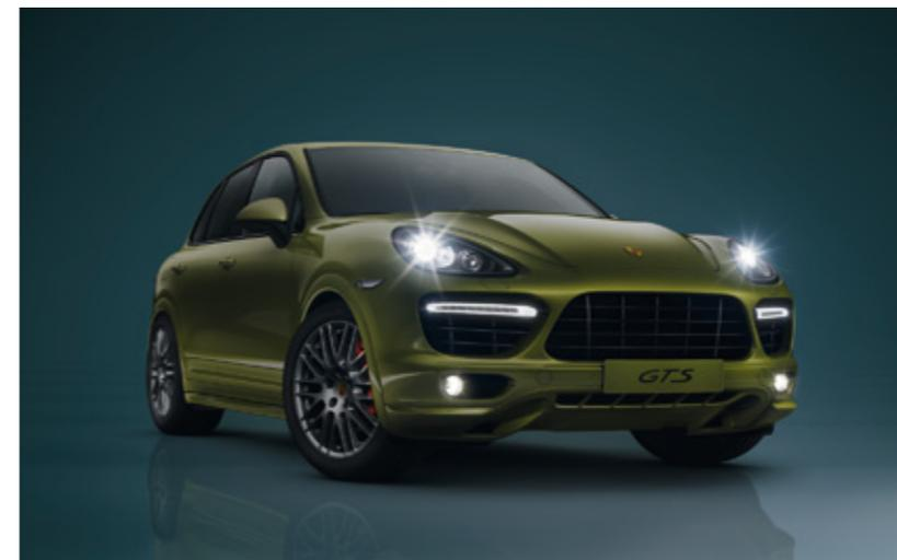
the static cornering lights activate the auxiliary headlights in order to illuminate more of the road in tight corners and turns.
