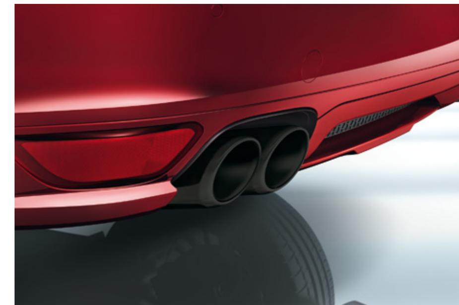
Sport exhaust system with twin dual-tube tailpipes trimmed in matte black
