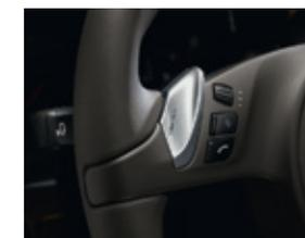
PDK gearshift switches on multifunction steering wheel
