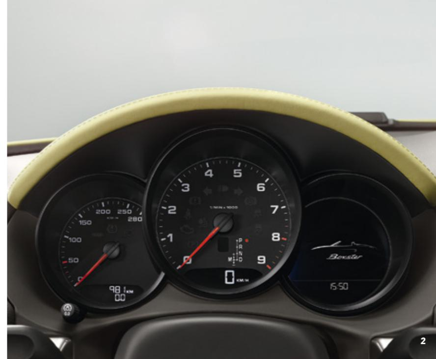
in minimalist black. The instrument on the left contains the analogue speedometer with digital trip meter and total distance display.
