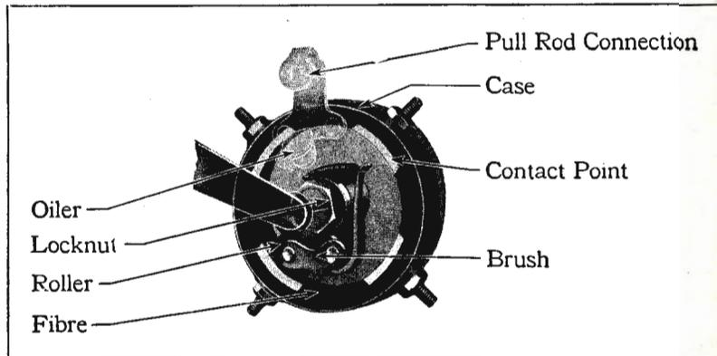
connected with a coil unit, an electrical circuit is passed through the entire system of primary wires. This circuit is only momentary, however, as the roller passes over the contact point very rapidly and sets up the circuit in each unit as the roller touches the contact point connected with that unit. The commutator should be kept clean and well oiled at all times.
