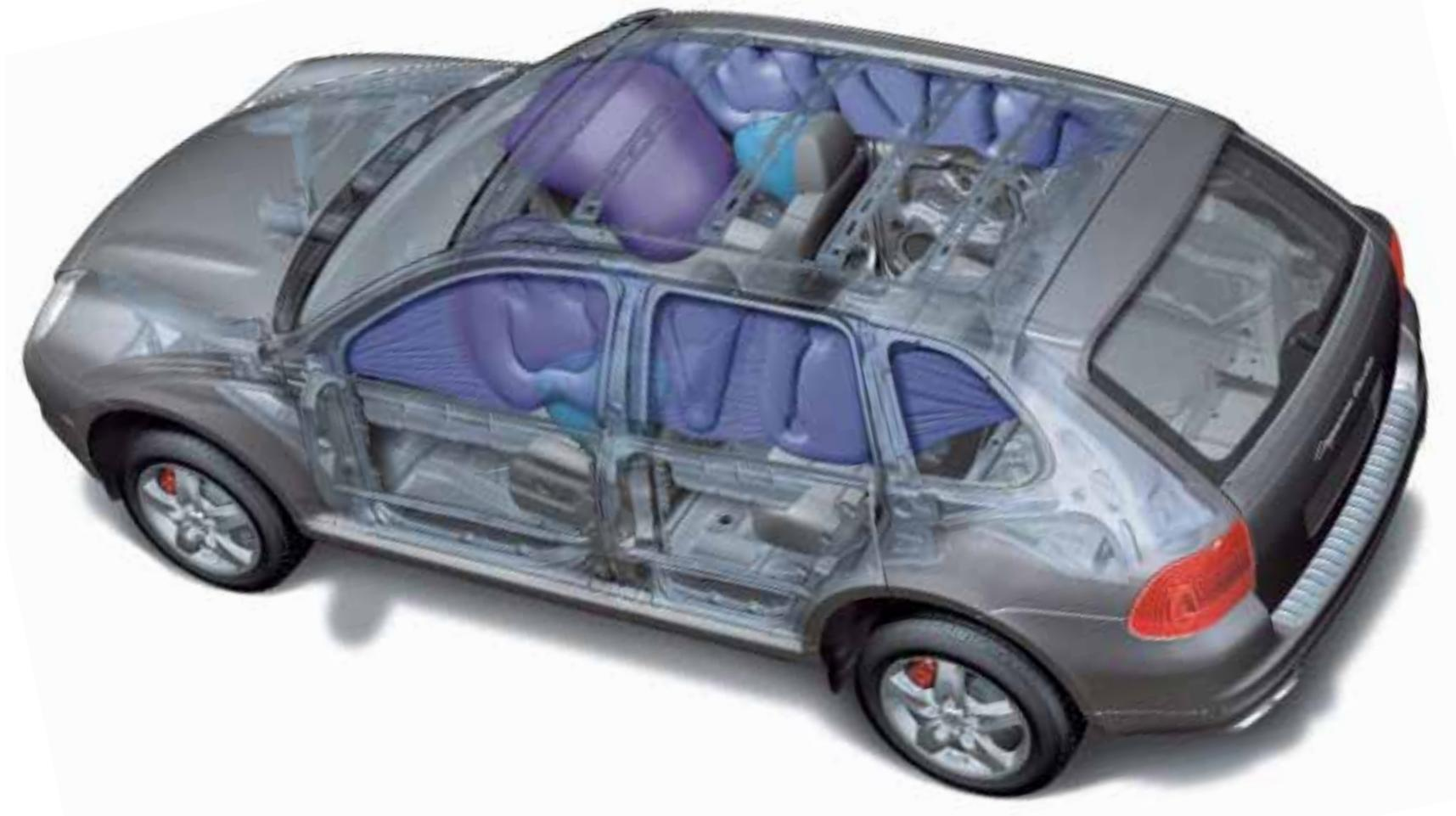
The Cayenne features two additional sensors at the front of the vehicle to detect head-on collisions. This allows deployment of the front airbags to be adapted to complex crash situations, thereby maximising protection.
