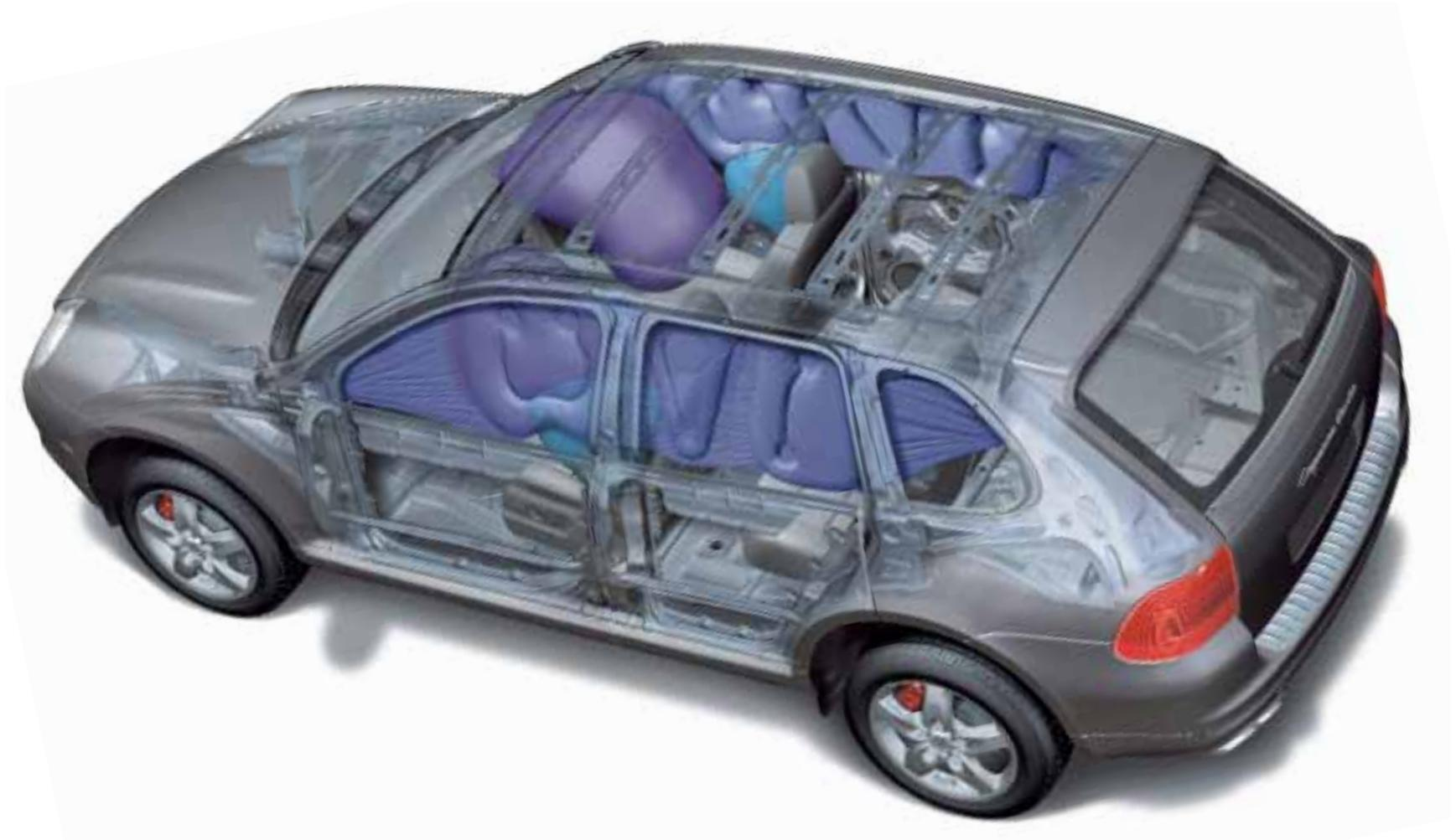
The Cayenne features two additional sensors at the front of the vehicle to detect head-on collisions. This allows deployment of the front airbags to be adapted to complex crash situations, thereby maximising protection.
