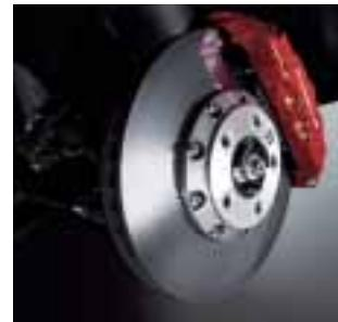
Power kit for Cayenne Turbo: 380 mm two-piece brake disc on the front axle
