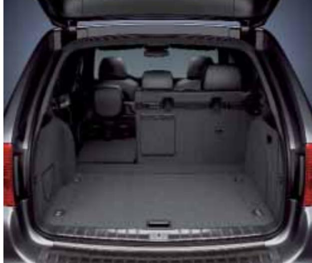
Smaller section of rear seat backrest folded (40% to 60%). Load space cover and luggage net removed.
