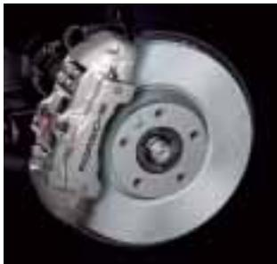
Standard brakes on Cayenne S: 350 mm disc brake on the front axle
