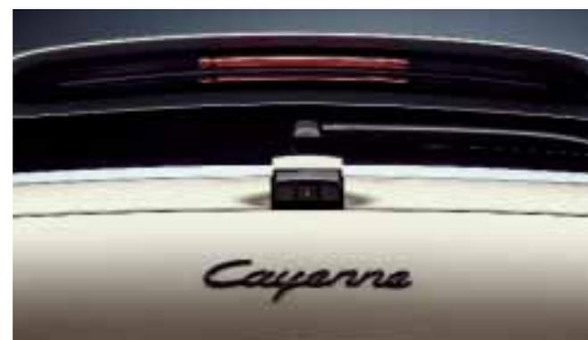
Reversing camera deployed
