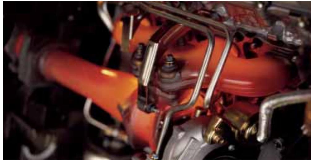
Cayenne turbocharged engine, turbocharger
