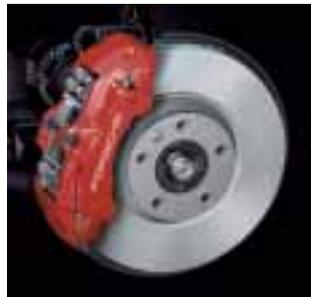
Standard brakes on Cayenne Turbo: 350 mm disc brake on the front axle
