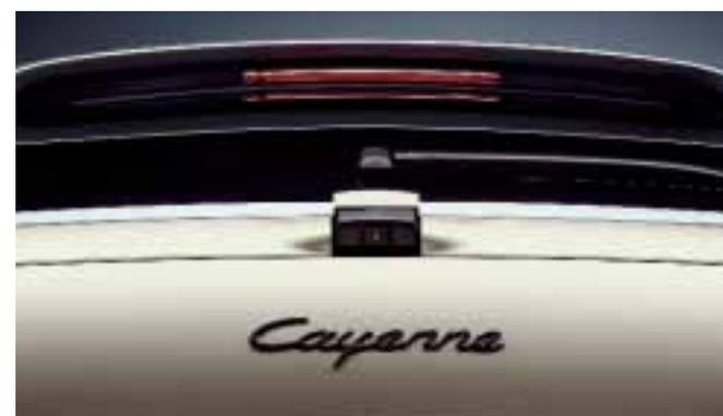
Reversing camera deployed
