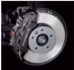
Standard brakes on Cayenne: 330 mm disc brake on the front axle
