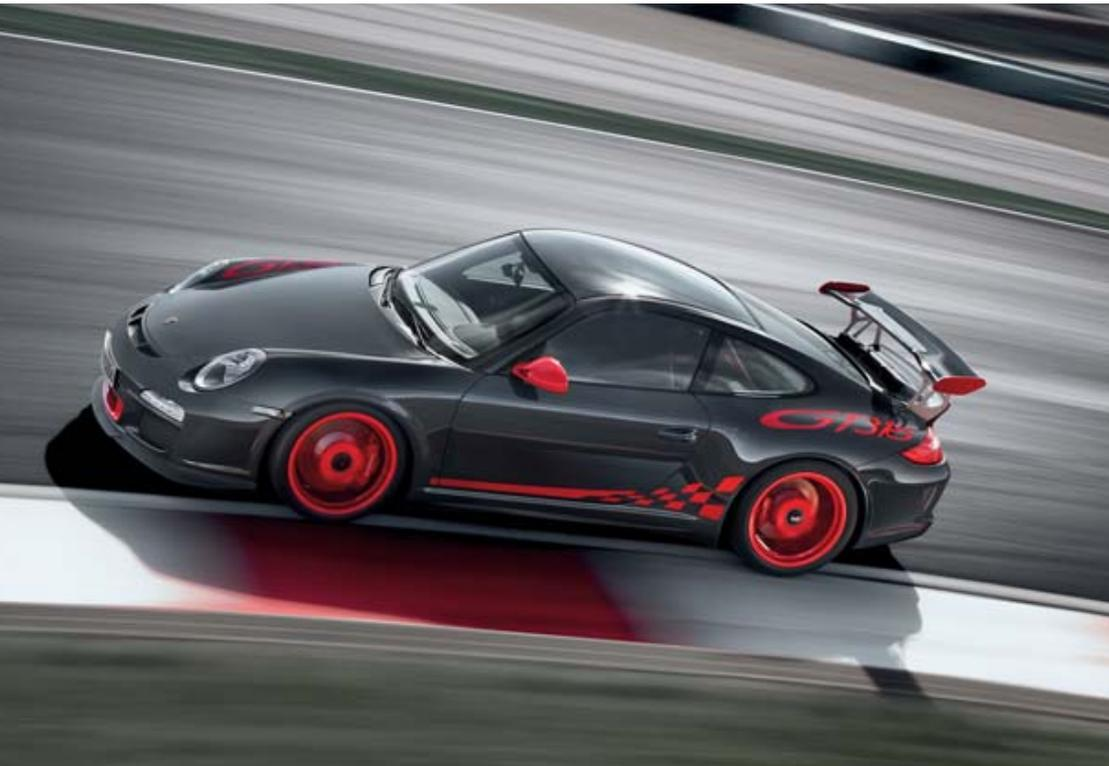
including titanium, aluminium and carbon. The new 911 GT3 RS also has lightweight door panels and a rear window made from a synthetic material. For use on the racetrack, for the first time Porsche is offering an optional lithium-ion battery (page 75), thus saving another 10 kg.
