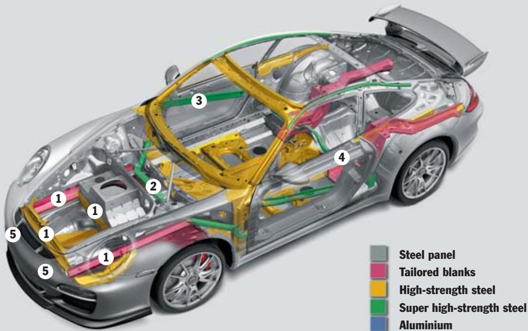
minor collision, a system of easily replaceable impact absorbers (5) prevents more serious damage.
