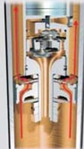
Left: Compression in 'Normal' mode – damper piston and bypass valve
