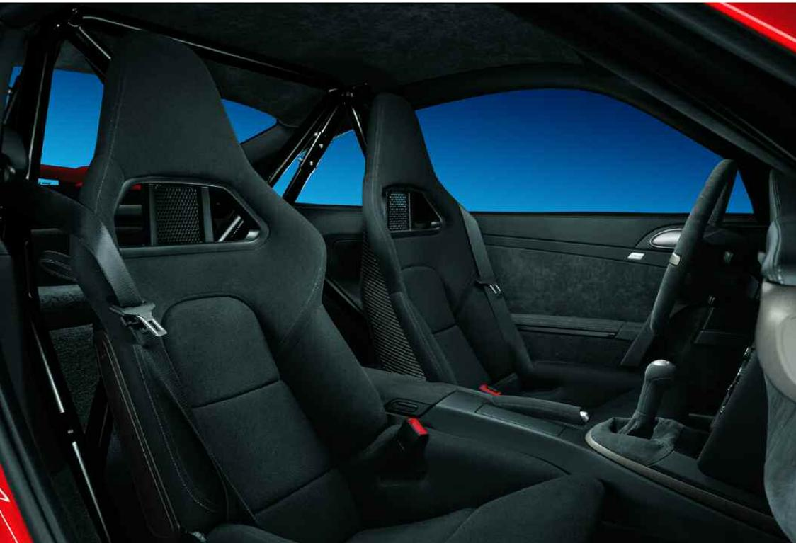
It consists of a roll cage that is bolted to the body behind the front seats, a six-point racing harness in red for the driver's side, a fire extinguisher with mounting bracket and preparation for a battery master switch.
