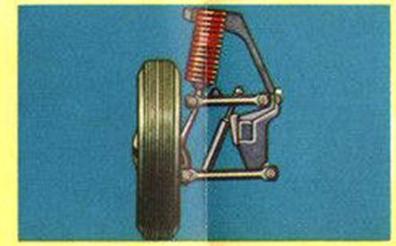
Long Coil Springs and rubber pillows, teamed with improved aerotype shock absorbers, softly smother road roughness and noise.
