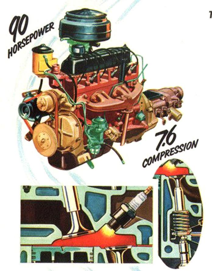
F-Head Design provides full downward flow of fuel mixture, together with a controlled combustionchamber turbulence for highest efficiency combustion and with less susceptibility to carbon. Selfcleaning exhaust valve postpones grinding for thousands of miles.
