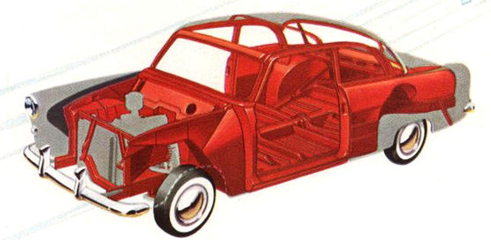
Willys Aero-Frame Construction eliminates needless weight and produces a car structure that is rig-
