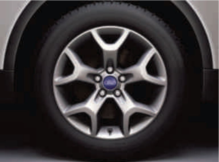
Alloy wheel – 17", 5x2-spoke, 235/55 tyres. (Standard on Zetec)
