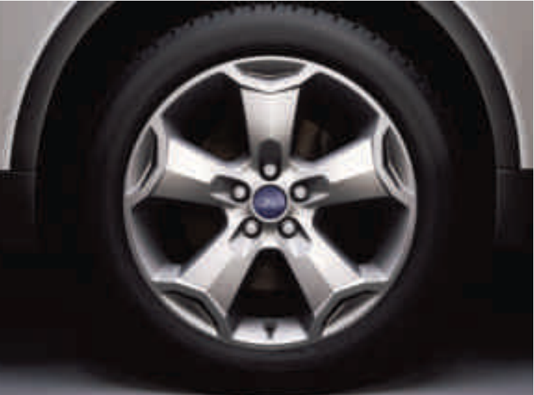
Alloy wheel – 7.5x17", 5x2-spoke, 235/55 tyres. (Standard on Titanium)
