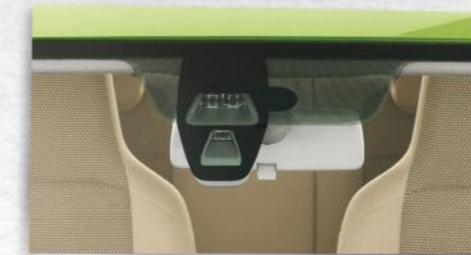
Citigo also features advanced technology - an optional 'City-safe' brake assist sensor that monitors the area in front of the vehicle, actively assisting braking at speeds below 19 mph when there is danger of a collision. Please note that it is the driver's responsibility to be in control of the vehicle at all times.
