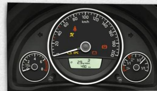
On all Citigo models the central feature is a **large speedometer**. The SE, Sport and Elegance dials (shown here) also feature a **rev counter** and a **fuel gauge**. S models features a digital fuel gauge.
