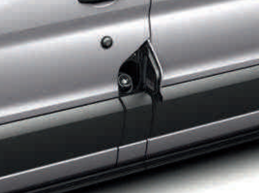
Ford Easy-Fuel capless refuelling system (Standard)
