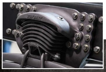
The hollows in the rubber center pivot of the TufTrac 2-Stage provide a smoother ride when driving unladen.
