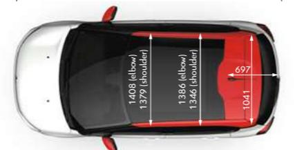
\* Vehicle width/width with slide mirrors out. All measurements are in millimetres.
