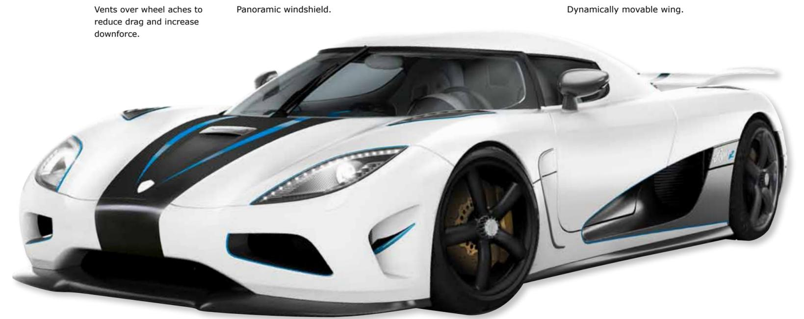
Vents over wheel arches to reduce drag and increase downforce.
