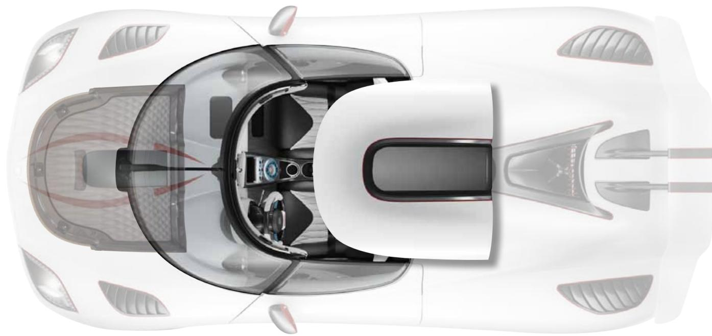
The roof is easily removed and it is designed to stow away perfectly in the front luggage compartment. This unique and practical feature sets the Koenigsegg Agera R apart from all other hypercars.
