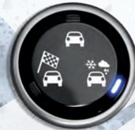
The Dynamic Selector Traction Control System lets you choose three distinct drive modes to promote confident driving. AUTO mode is calibrated for everyday driving. SPORT mode provides a quicker driving response and sportier handling. TRACTION+ mode maximizes low-speed traction on slippery and off-road surfaces.
