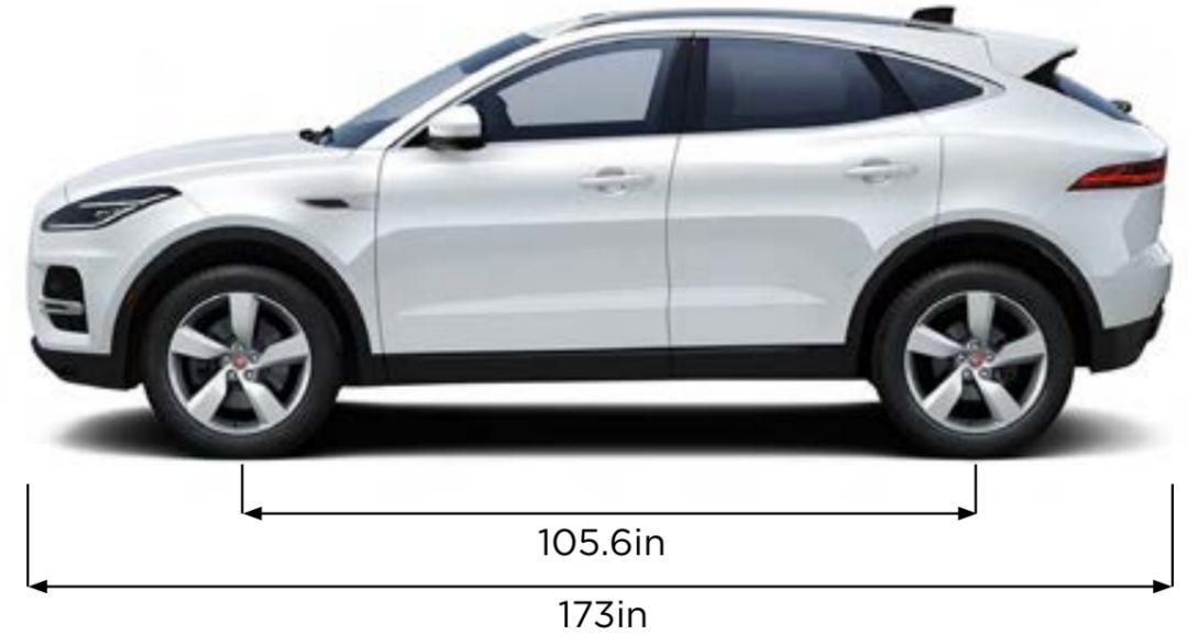
Dimensions were measured with vehicle at unladen weight.
